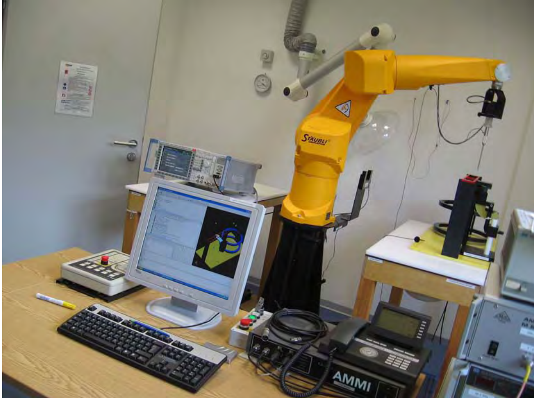
Photo 2: Probe calibration within Helmholtz coil before measurement
