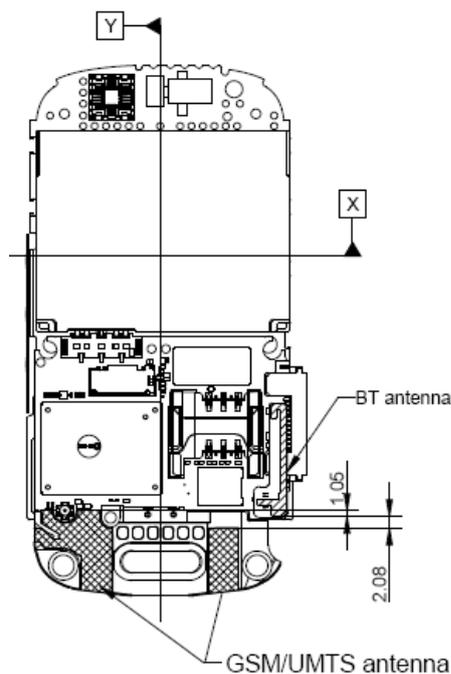
The output power of BT antenna is 4.3mW. According to the SAR measurement results and the distance between the two antennas, we can draw the conclusion that: stand-alone SAR and simultaneous transmission SAR are not required for BT transmitter, because the all SAR measurement results of GSM transmitter are <1.2W/kg and BT antenna is <2.5cm from other antenna.
