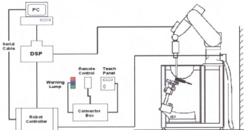
**Picture 1: SAR Lab Test Measurement Set-up**
