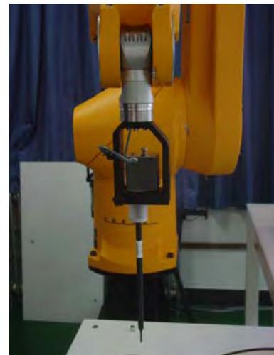
**Picture3:ES3DV3 E-field probe**
