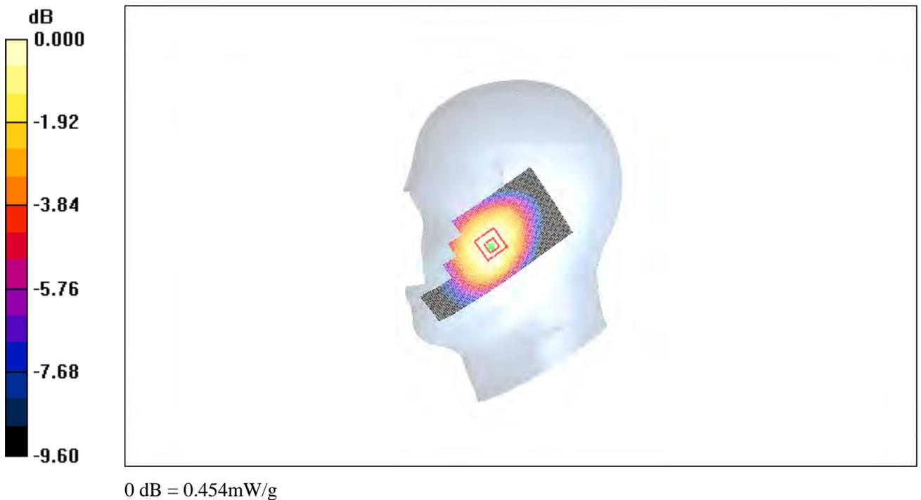
**Fig. 11 850 MHz CH128 – Slide up**
