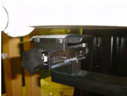
DUT position towards the body, 15 mm distance
