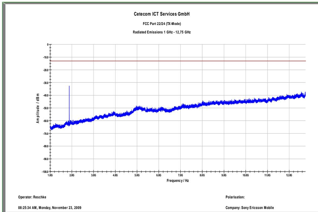
Carrier suppressed with a rejection filter
