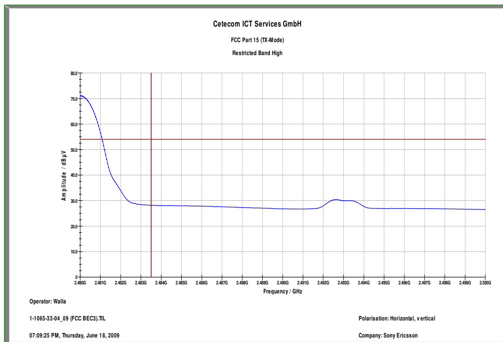
Plot 1: Band edge compliance at the highest channel with far away emissions
