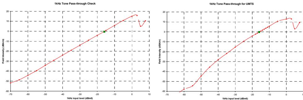
This model was verified to be within the linear region for ABM1 measurements at -16 dBm0. This measurement was taken in the axial configuration above the maximum location, cellular band, mid channel.
