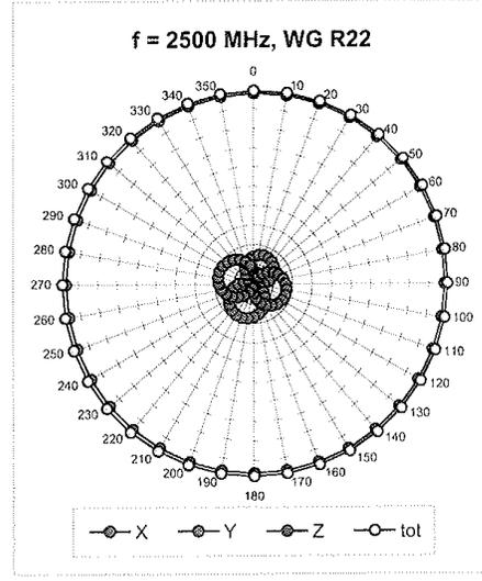
Receiving Pattern ( $\phi$ ),  $\vartheta = 0^\circ$
