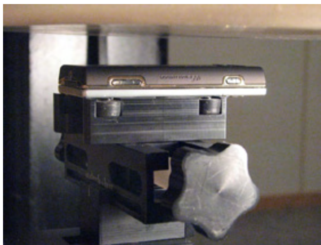
DUT position towards the body with a distance of 15 mm
