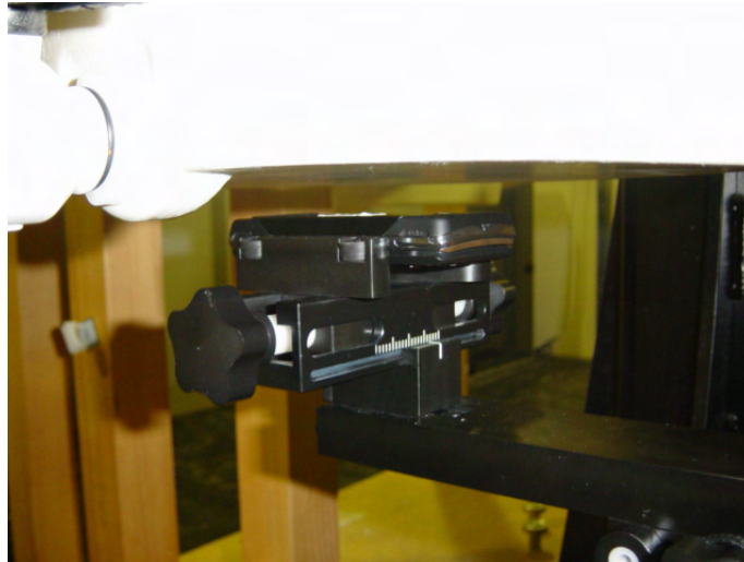
DUT in body position with 15 mm distance
