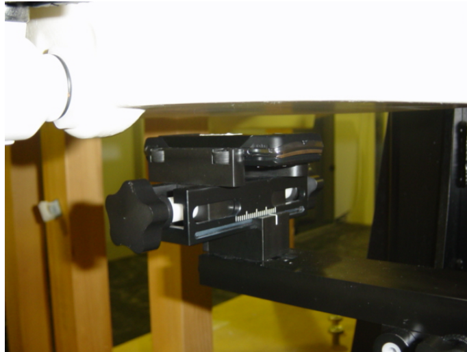
DUT in body position with 15 mm distance
