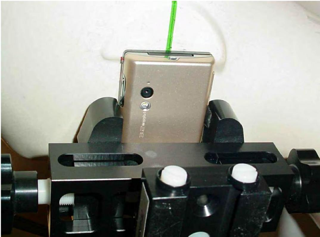
Photo 15: Test position left hand tilted 15° (slide in)
