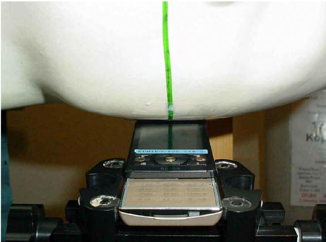
Photo 21: Test position left hand tilted 15° (slide opened)
