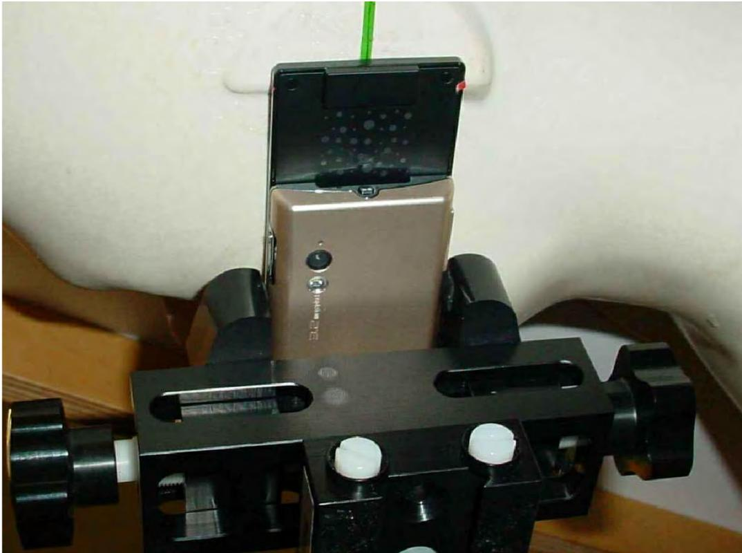
Photo 20: Test position left hand tilted 15° (slide opened)
