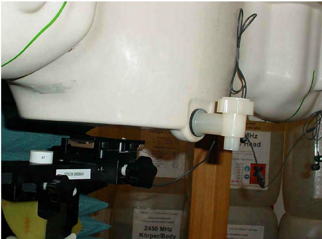
Photo 33: Test position body worn front side with 15 mm distance
