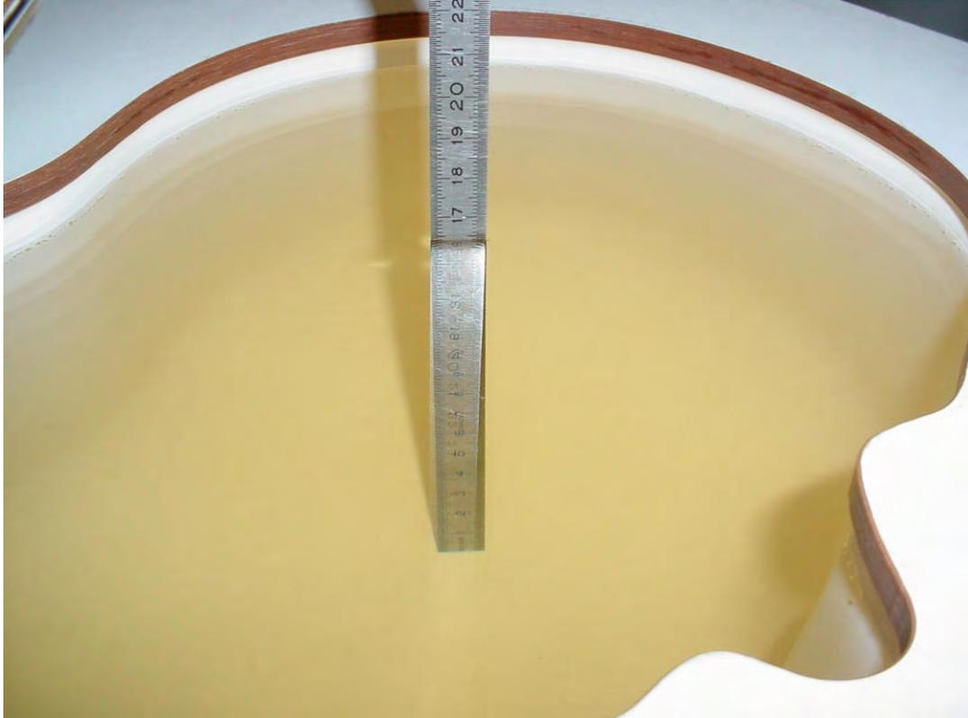
Photo 37: Liquid depth 850 MHz body simulating liquid
