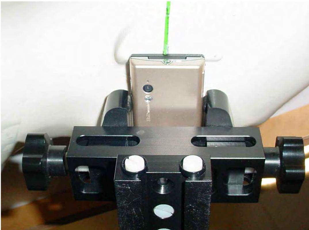
Photo 25: Test position right hand tilted 15° (slide in)
