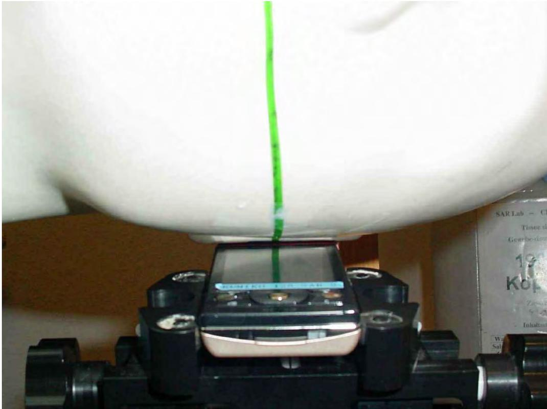
Photo 16: Test position left hand tilted 15° (slide in)
