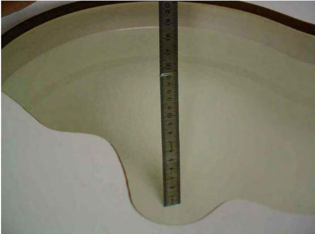
Photo 39: Liquid depth 1900 MHz body simulating liquid
