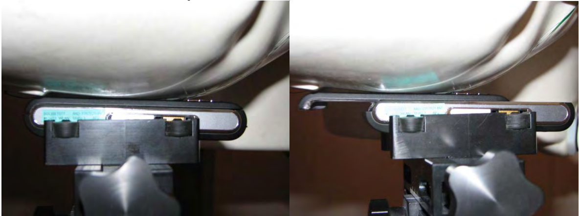
DUT position towards the head: Cheek close and open(touch) position
