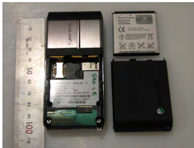
Battery and cover removed
