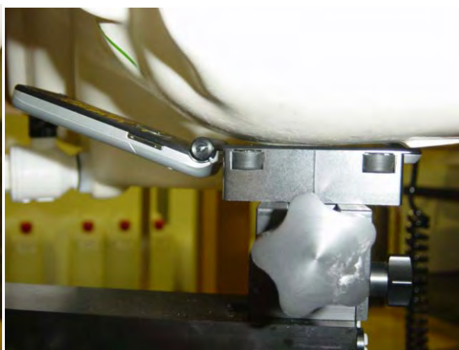
DUT position towards the head: Cheek (touch) position
