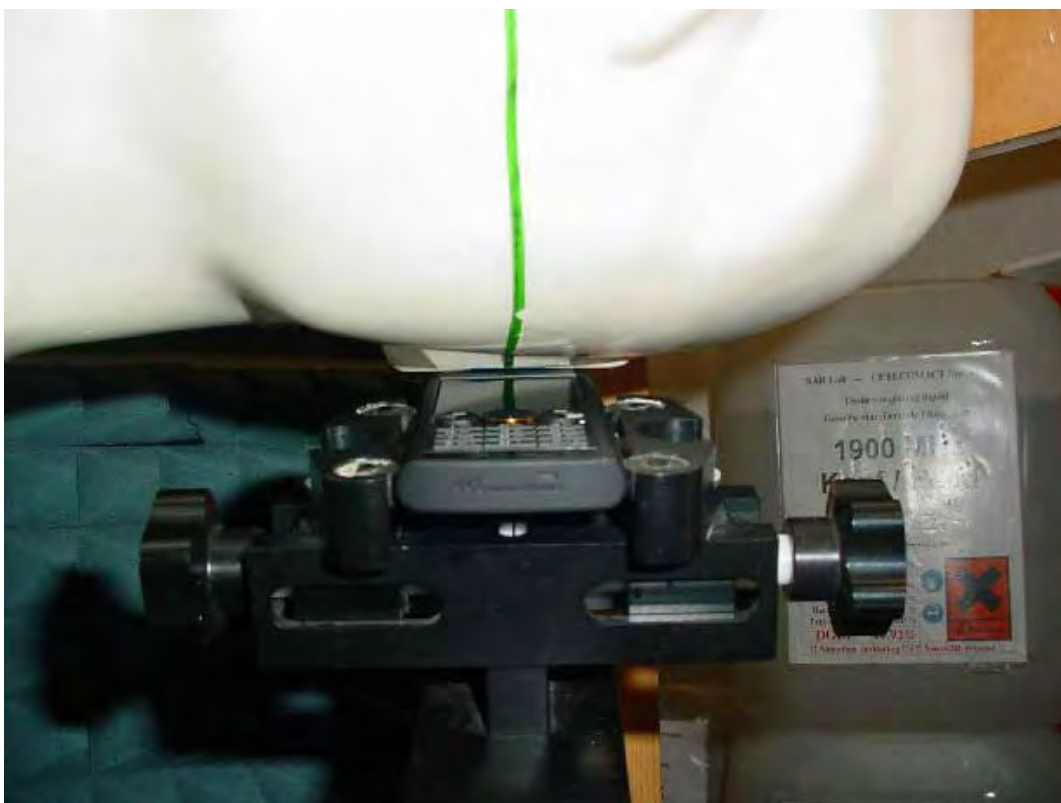
Photo 12: Test position left hand tilted 15°
