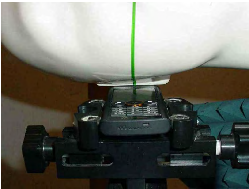
Photo 18: Test position right hand tilted 15°
