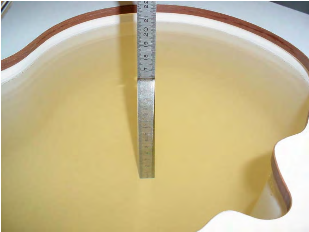
Photo 24: Liquid depth 850 MHz body simulating liquid
