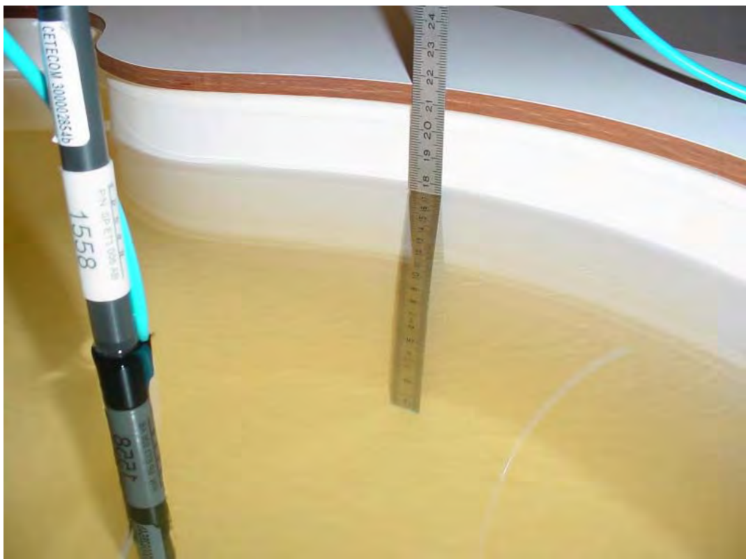
Photo 24: Liquid depth 850 MHz body simulating liquid
