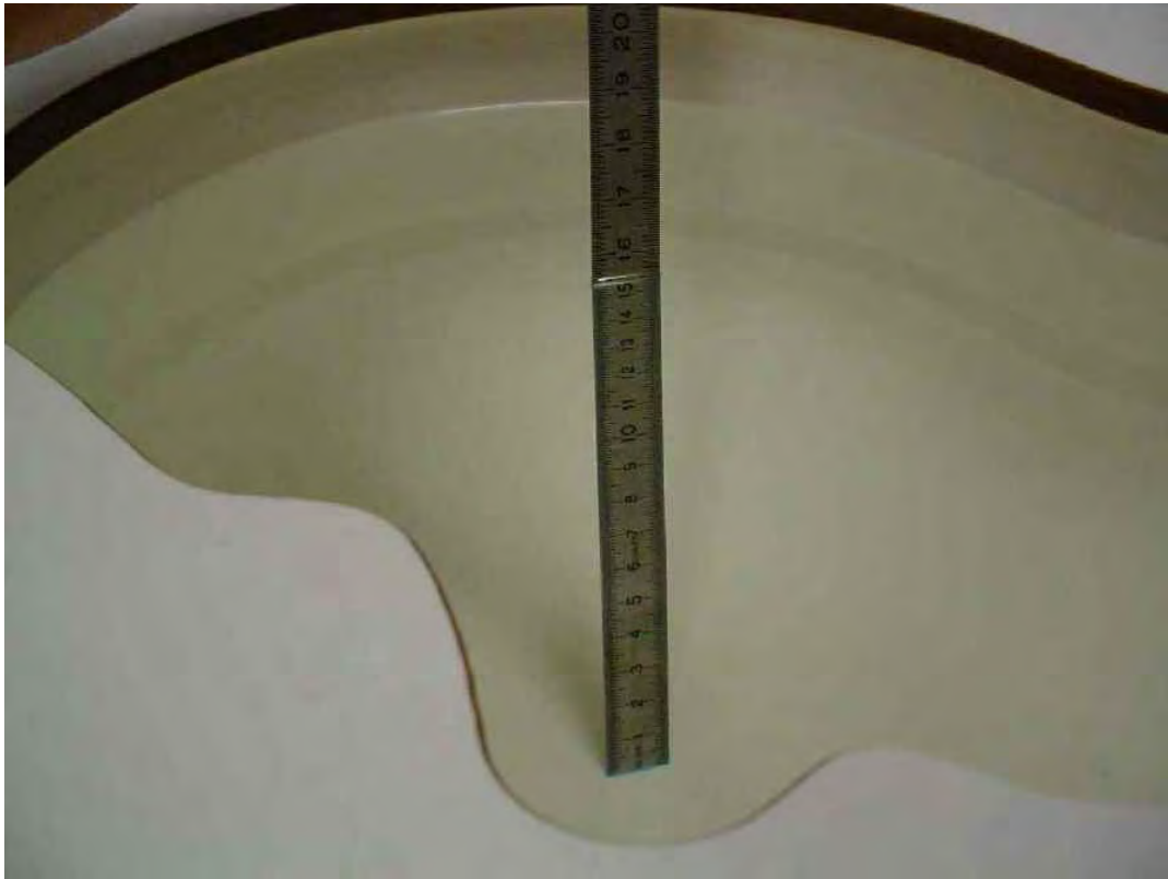
Photo 26: Liquid depth 1900 MHz body simulating liquid
