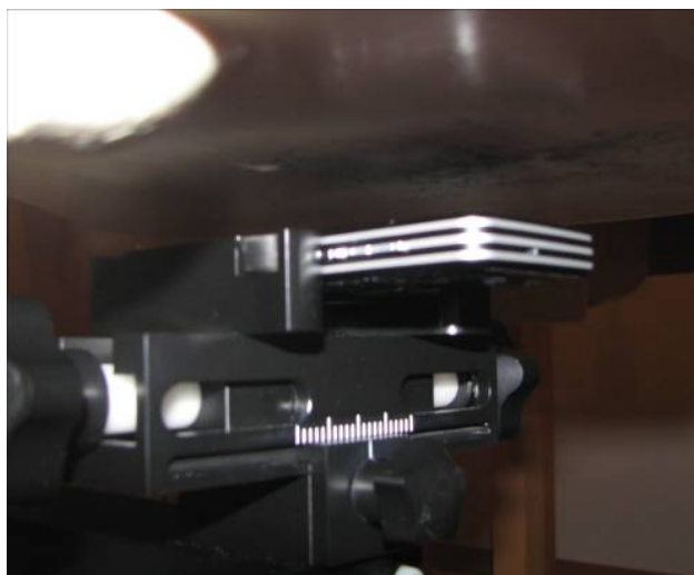
DUT in body position with 15 mm distance
