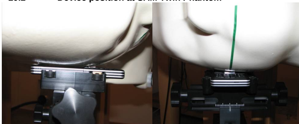
DUT position towards the head: Cheek (touch) position
