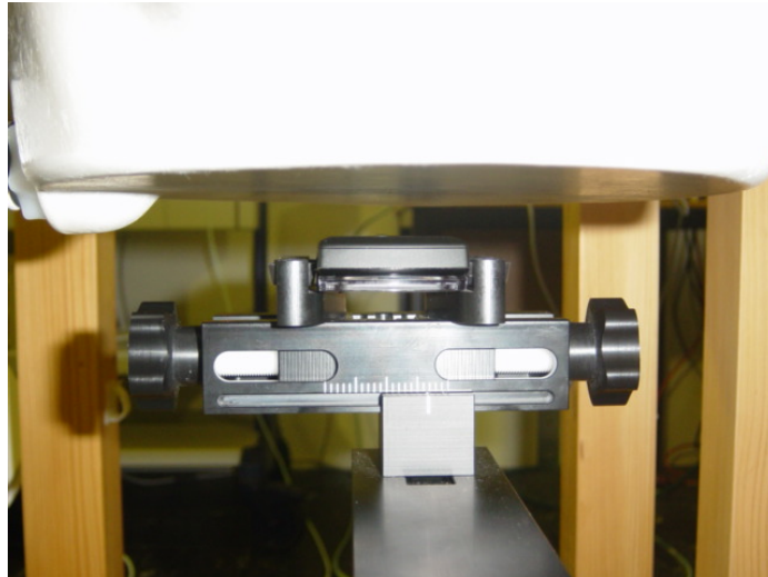
DUT in body position with 15 mm distance
