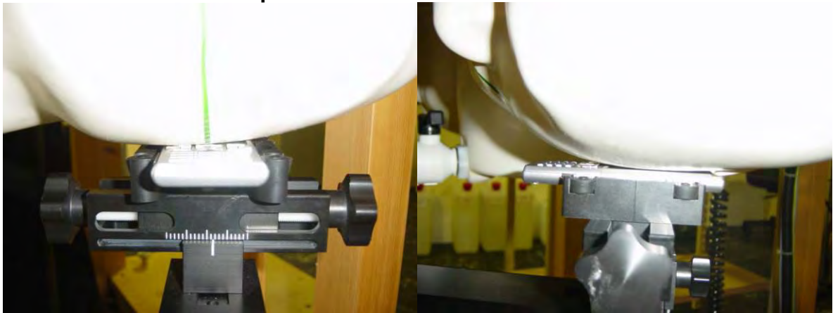
DUT position towards the head: Cheek (touch) position
