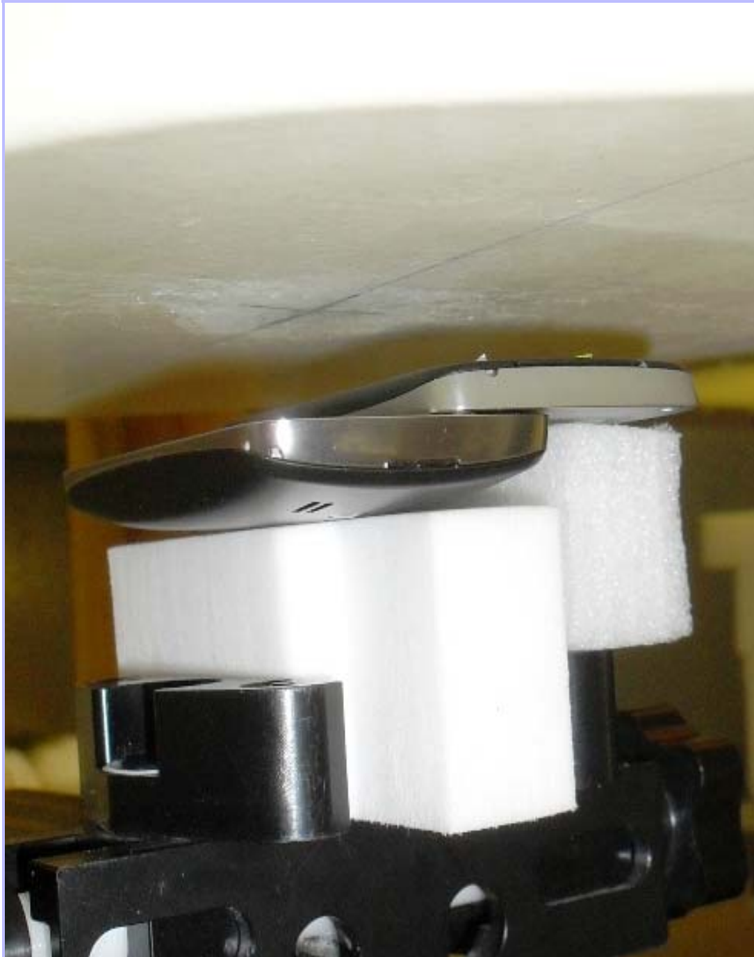
PHT/81152JD01/009: Front of EUT With Slide Open Facing Phantom
