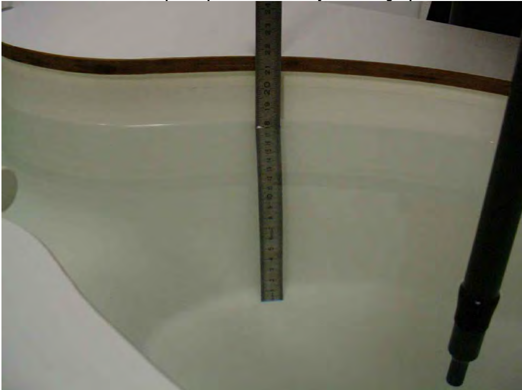
Photo 6: Liquid depth 2450 MHz body simulating liquid
