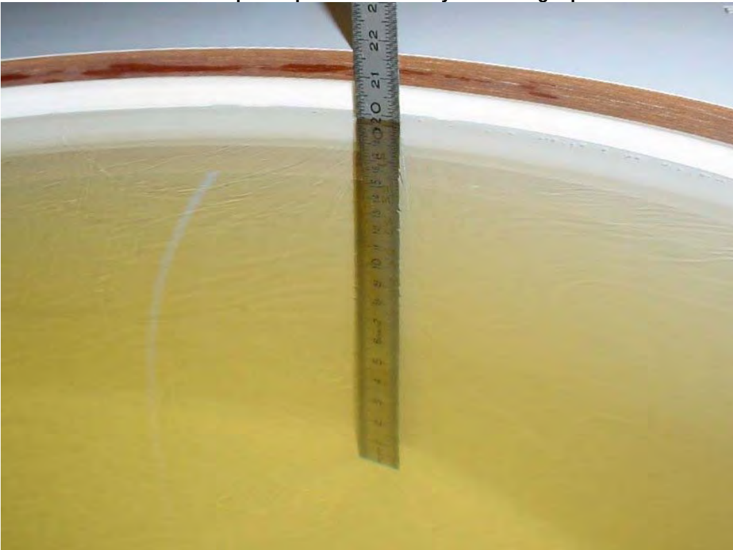
Photo 2: Liquid depth 850 MHz body simulating liquid
