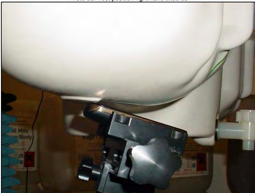
Photo 18: Test position right hand tilted 15°
