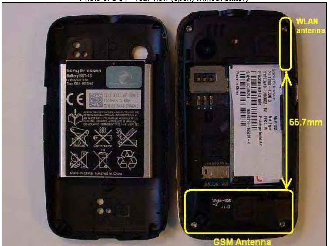
Photo 6: DUT - rear view (open) without battery
