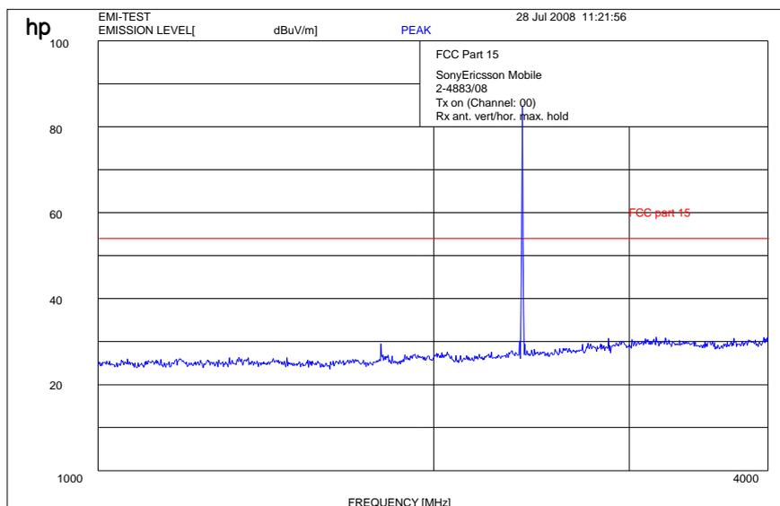
Plot 3: 4 - 12 GHz vertical/horizontal (lowest channel)
