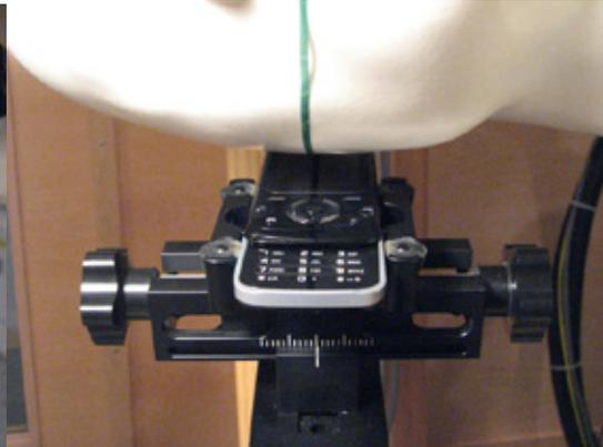
*DUT position towards the head: Tilt (touch + 15°) position open*
