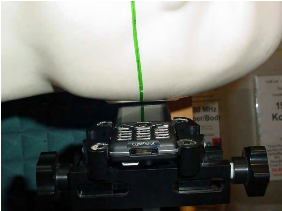
Photo 12: Test position left hand tilted 15°
