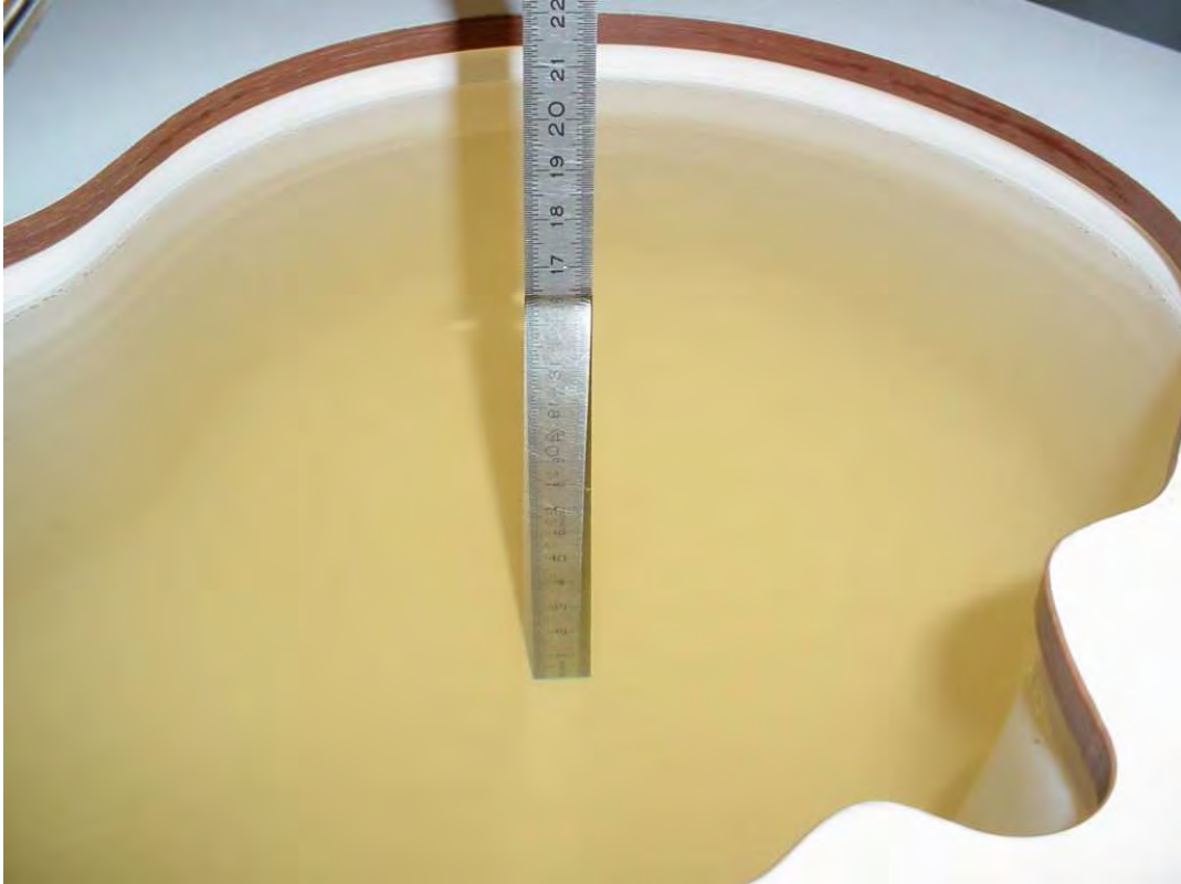
Photo 24: Liquid depth 850 MHz body simulating liquid
