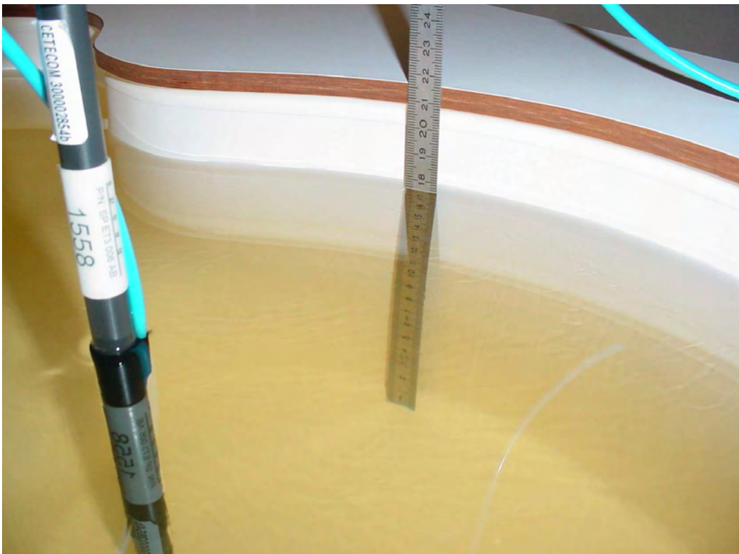
Photo 24: Liquid depth 850 MHz body simulating liquid
