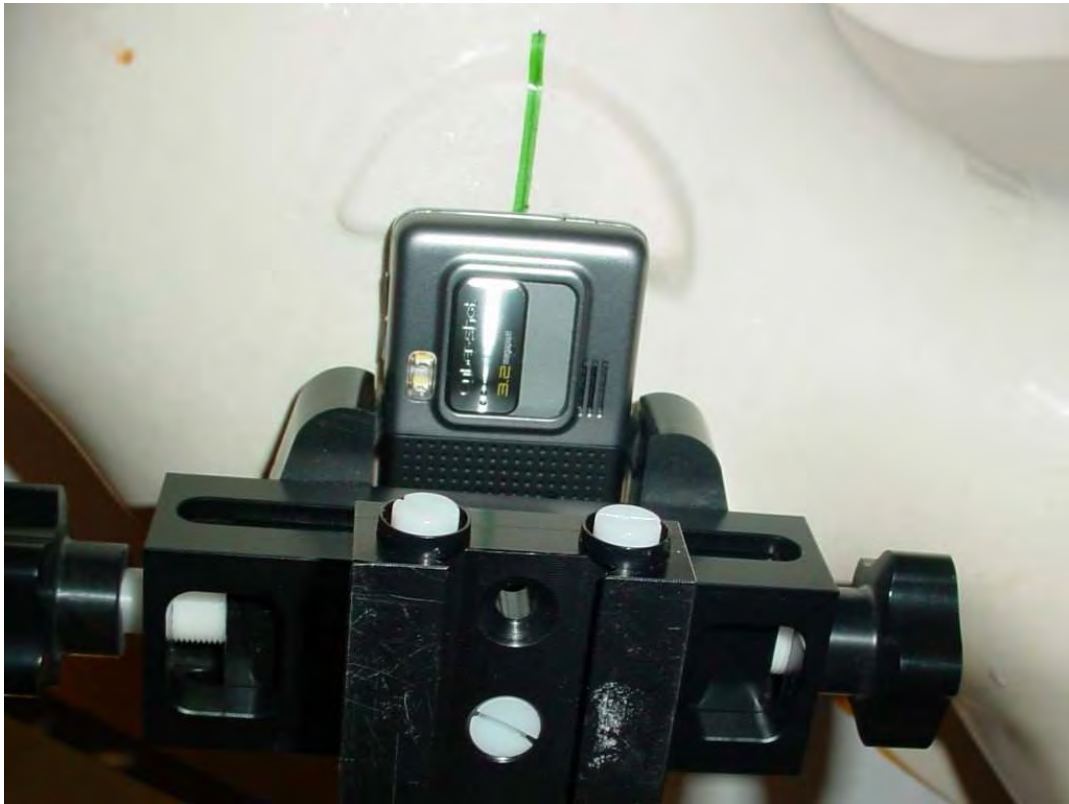
Photo 12: Test position left hand tilted 15°
