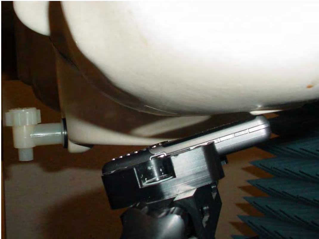
Photo 14: Test position right hand touched
