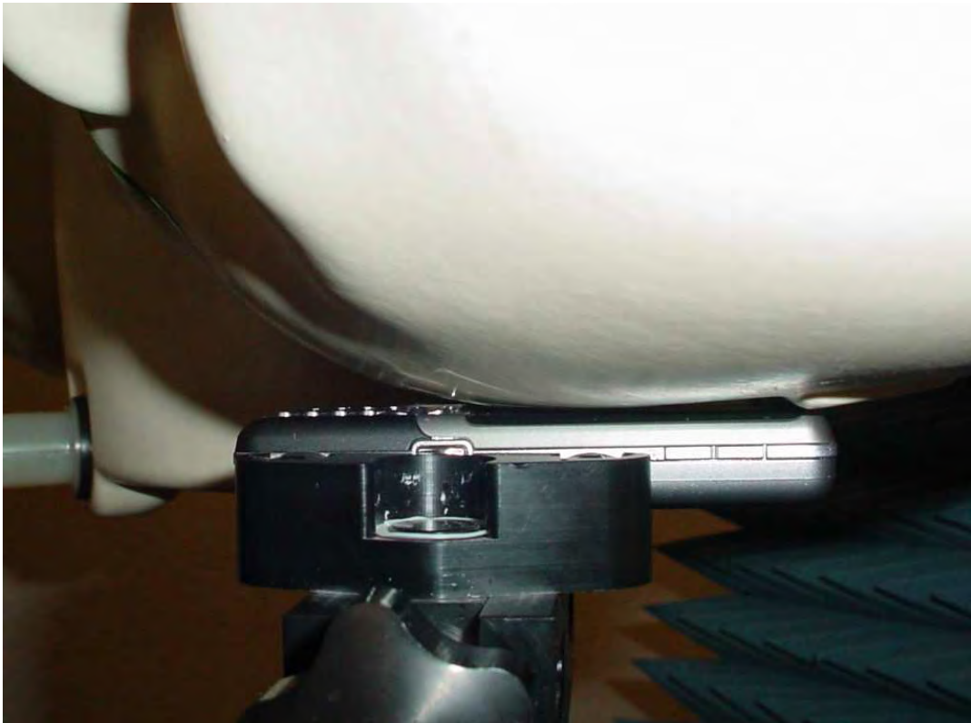
Photo 10: Test position left hand touched
