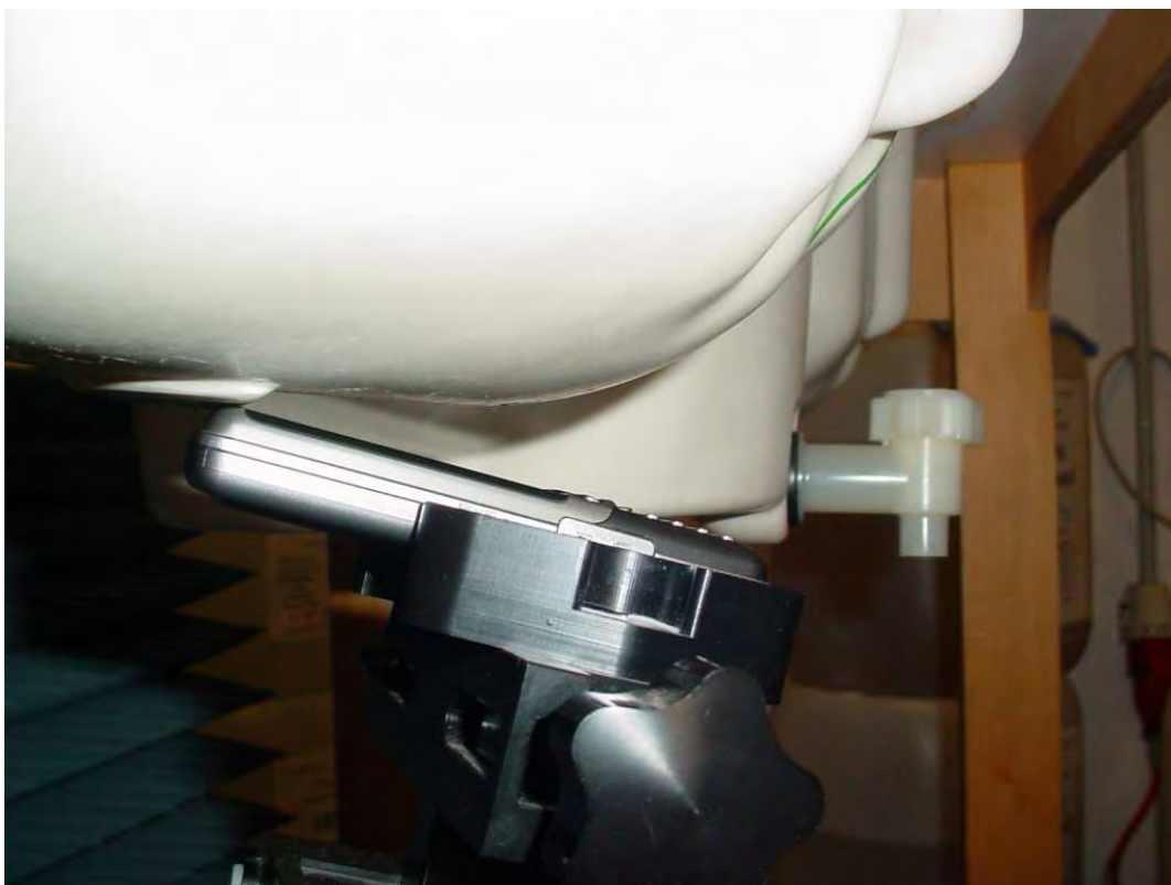
Photo 18: Test position right hand tilted 15°
