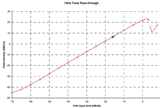
This model was verified to be within the linear region for ABM1 measurements. This measurement was taken in the axial ABM1 configuration above the maximum location in Table 6-3.
