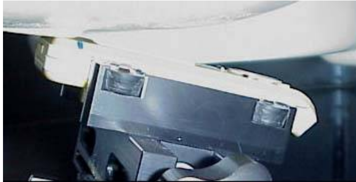
Position of device against head phantom using the "tilt" position
