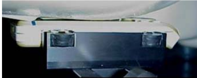
Position of device against head phantom using the “cheek” position
