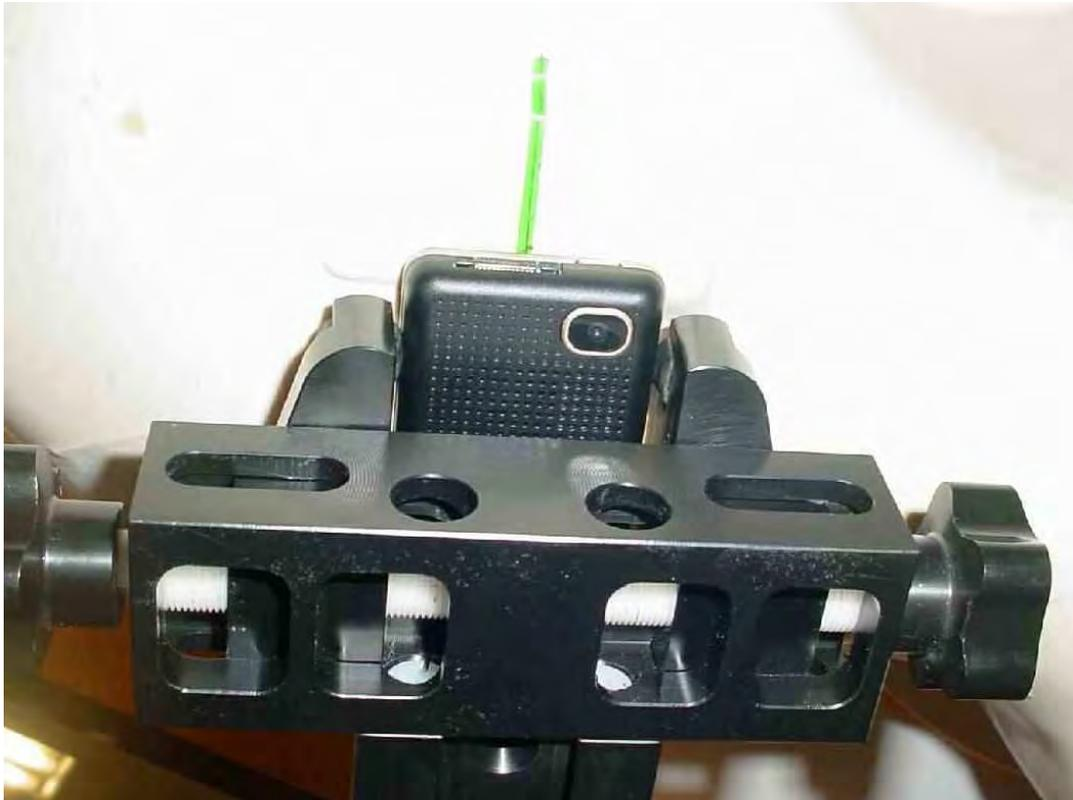
Photo 12: Test position left hand tilted 15°
