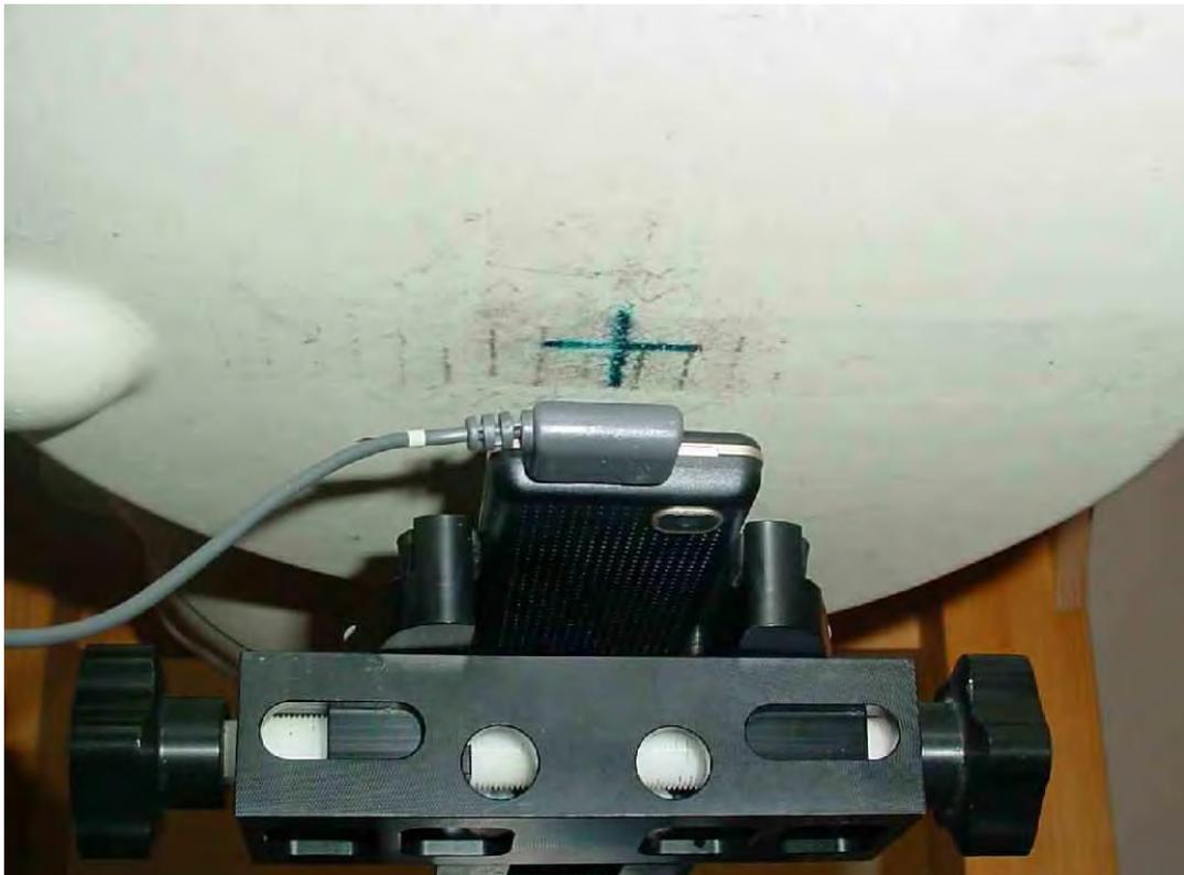
Photo 21: Test position body worn rear side (distance 15 mm)
