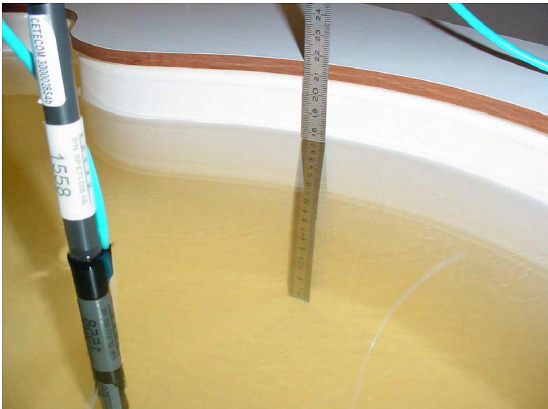
Photo 25: Liquid depth 1900 MHz head simulating liquid
