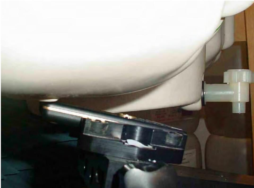
Photo 19: Test position body worn front side (distance 15 mm)
