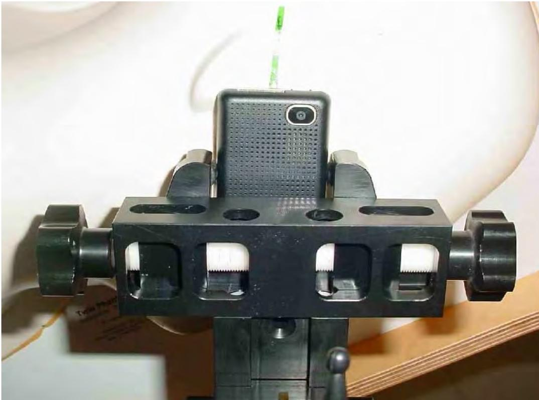
Photo 17: Test position right hand tilted 15°
