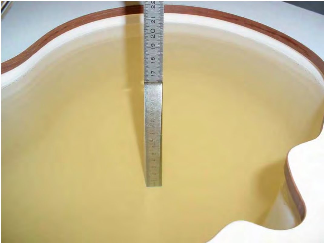
Photo 36: Liquid depth 850 MHz body simulating liquid
