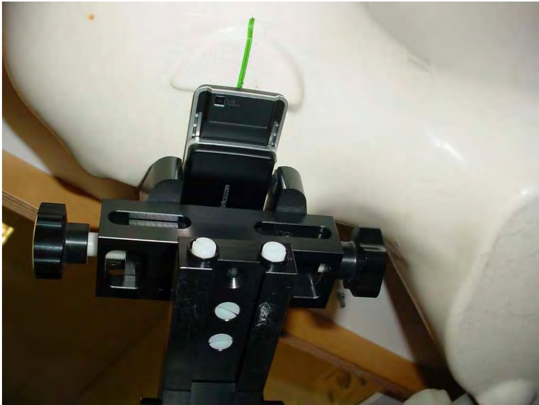
Photo 20: Test position left hand tilted 15° slide opened
