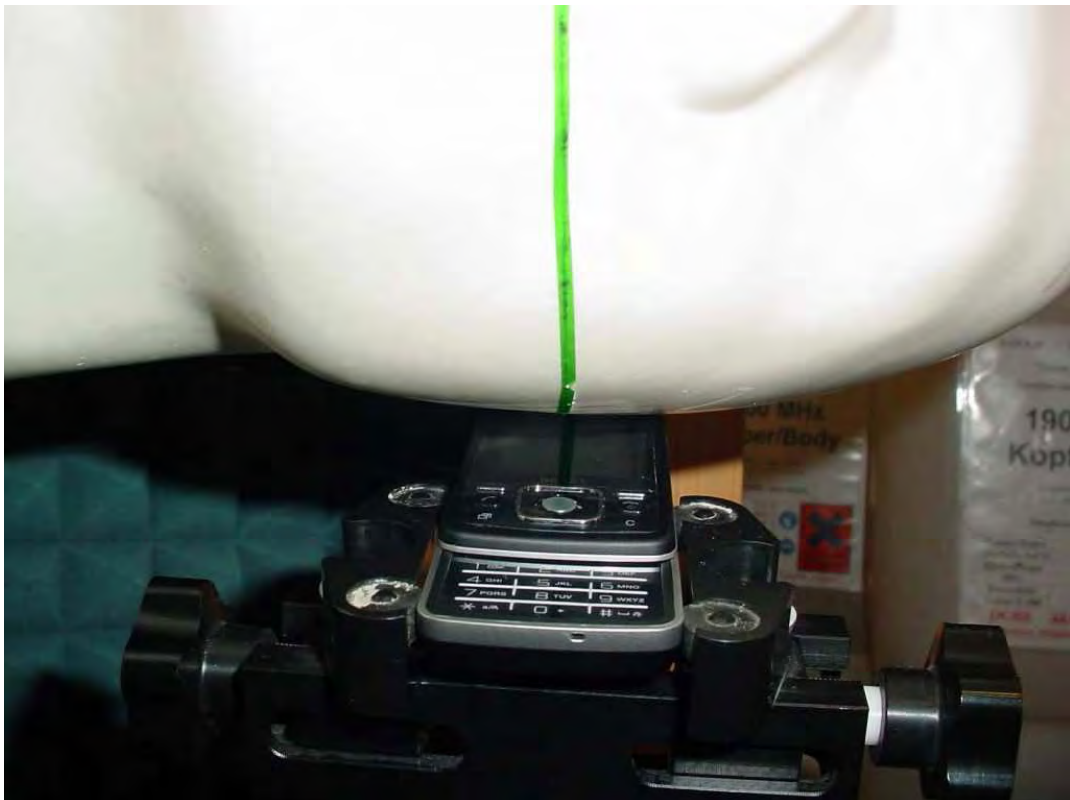
Photo 20: Test position left hand tilted 15° slide opened
