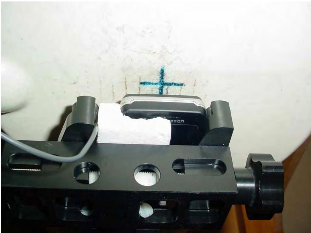
Photo 34: Test position body worn rear side (15 mm distance)
