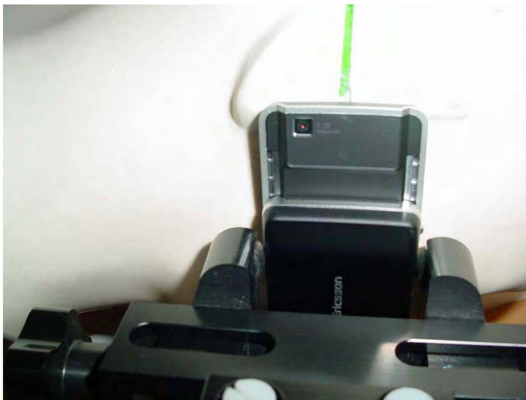
Photo 30: Test position right hand tilted 15° slide opened
