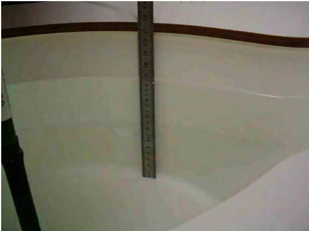
Photo 38: Liquid depth 1900 MHz body simulating liquid
