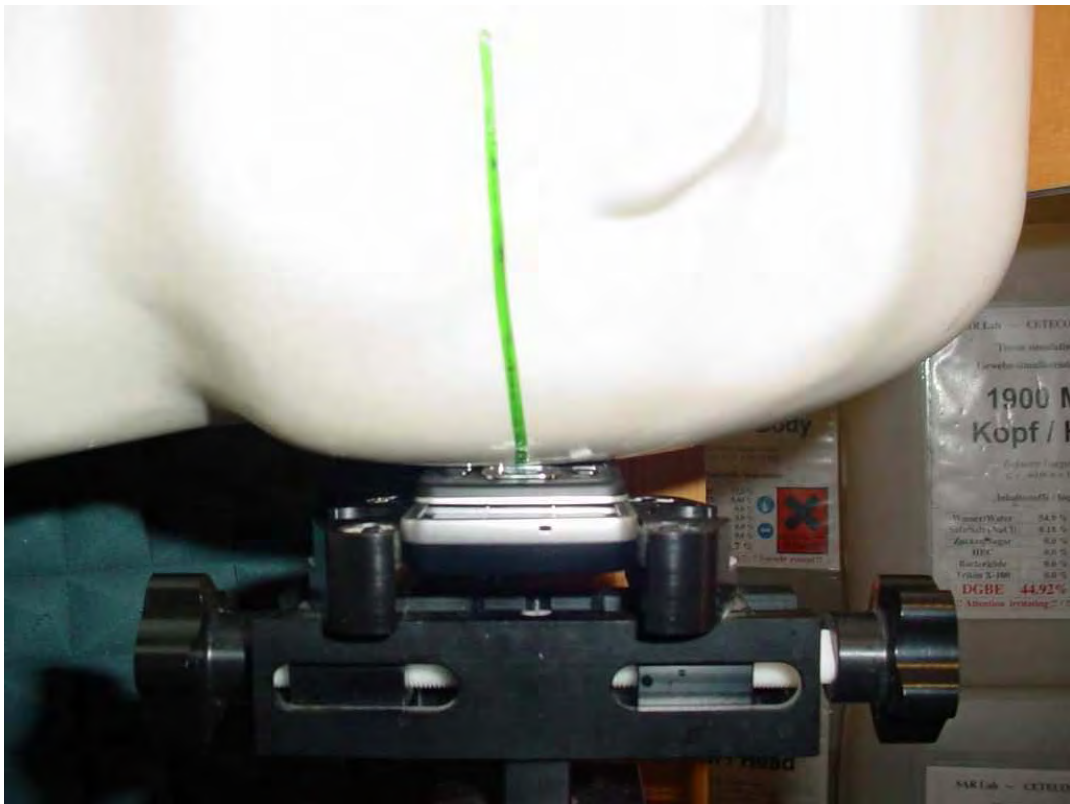
Photo 18: Test position left hand touched slide opened
