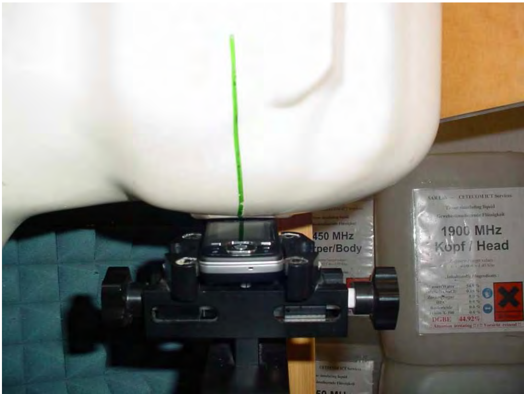
Photo 16: Test position left hand tilted 15°
