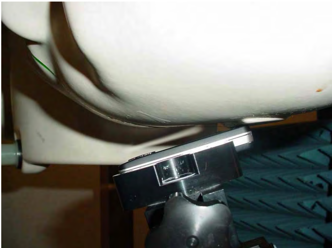
Photo 16: Test position left hand tilted 15°
