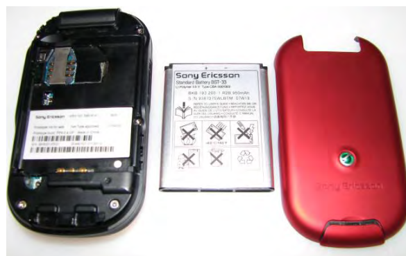
Battery and cover removed
