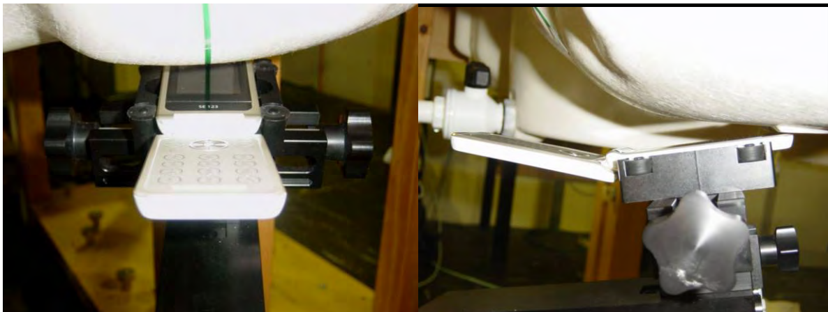
DUT position towards the head: Tilt (touch + 15°) position
