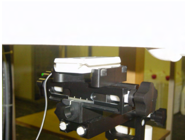
DUT in body position with 15 mm distance
