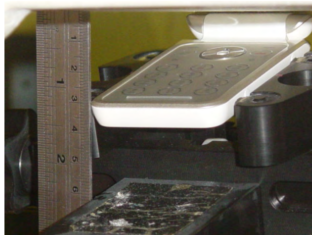
DUT position Head at Flat phantom 30mm
