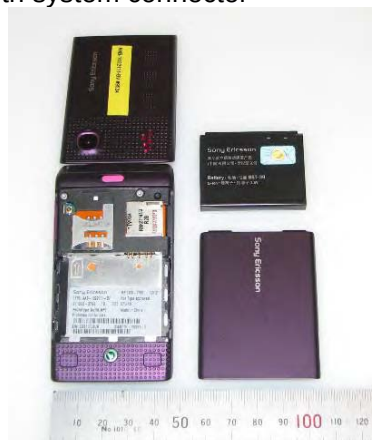
Battery and cover removed
