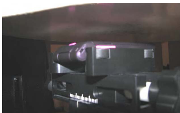
DUT in body position with 15 mm distance
