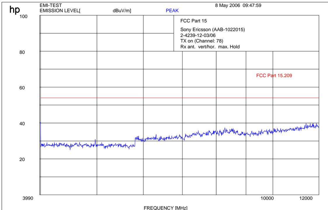
Plot : 12- 25 GHz vertical/horizontal (highest channel)
