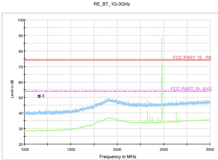
Fig.45. Radiated emission: GFSK, Channel 78, 1 GHz - 3 GHz
