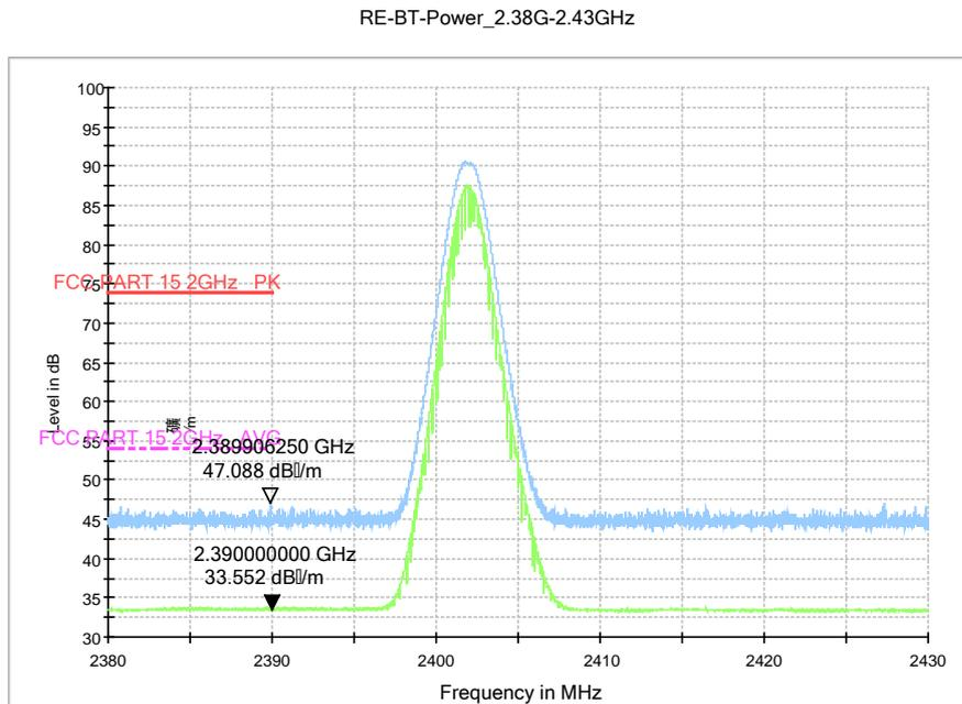
Fig.57. Radiated emission (Power):  $\pi/4$  DQPSK, low channel
