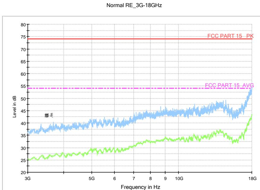
Fig.40. Radiated emission: GFSK, Channel 0, 3 GHz - 18 GHz
