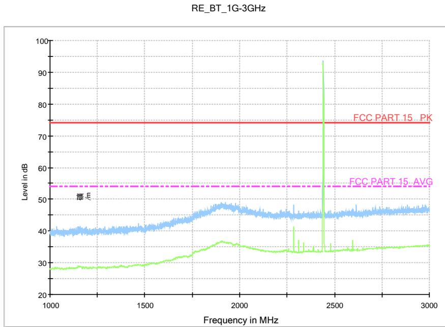
Fig.43. Radiated emission: GFSK, Channel 39, 1 GHz - 3 GHz
