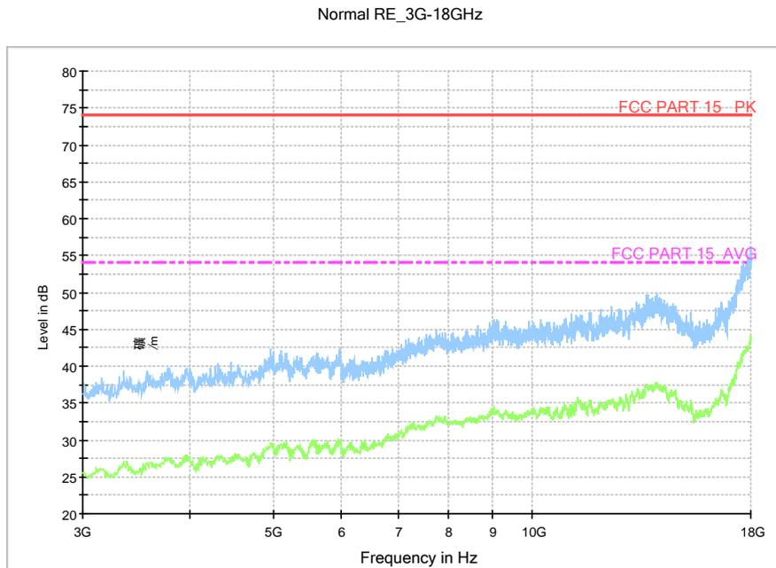
Fig.46. Radiated emission: GFSK, Channel 78, 3 GHz - 18 GHz
