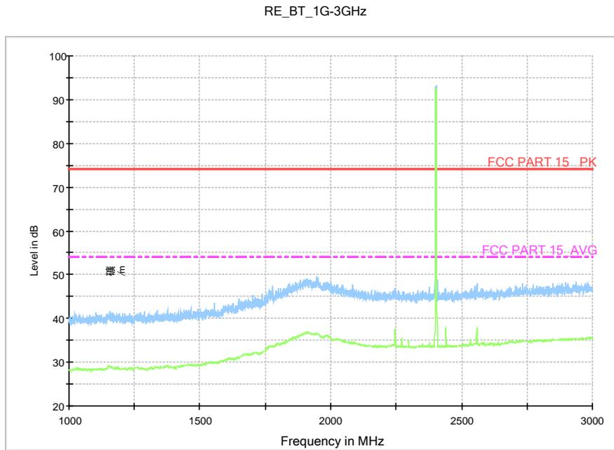
Fig.39. Radiated emission: GFSK, Channel 0, 1 GHz - 3 GHz
