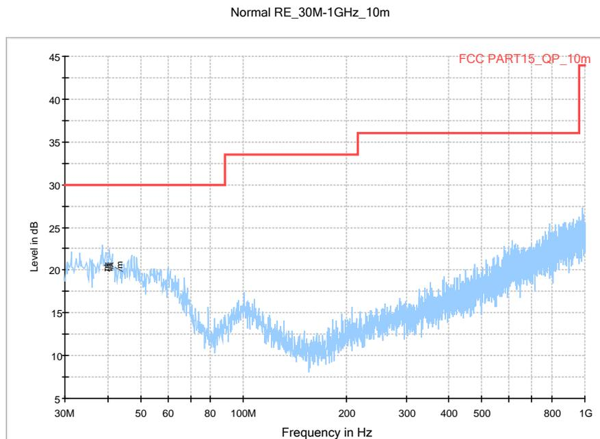
Fig.42. Radiated emission: GFSK, Channel 39, 30 MHz - 1 GHz
