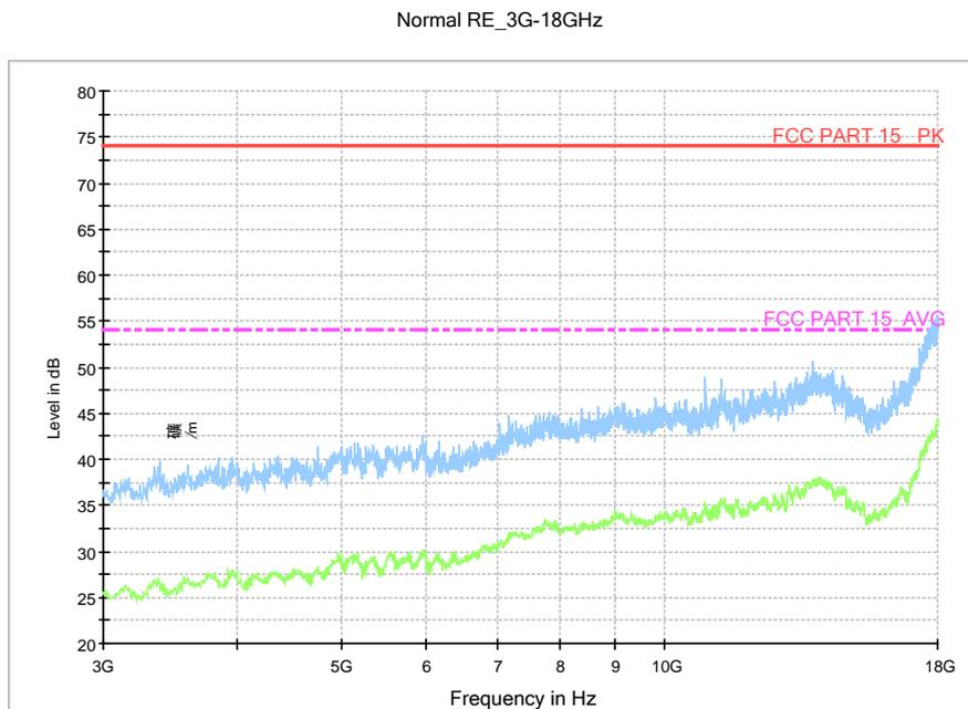
Fig.54. Radiated emission:  $\pi/4$  DQPSK, Channel 39, 3 GHz - 18 GHz
