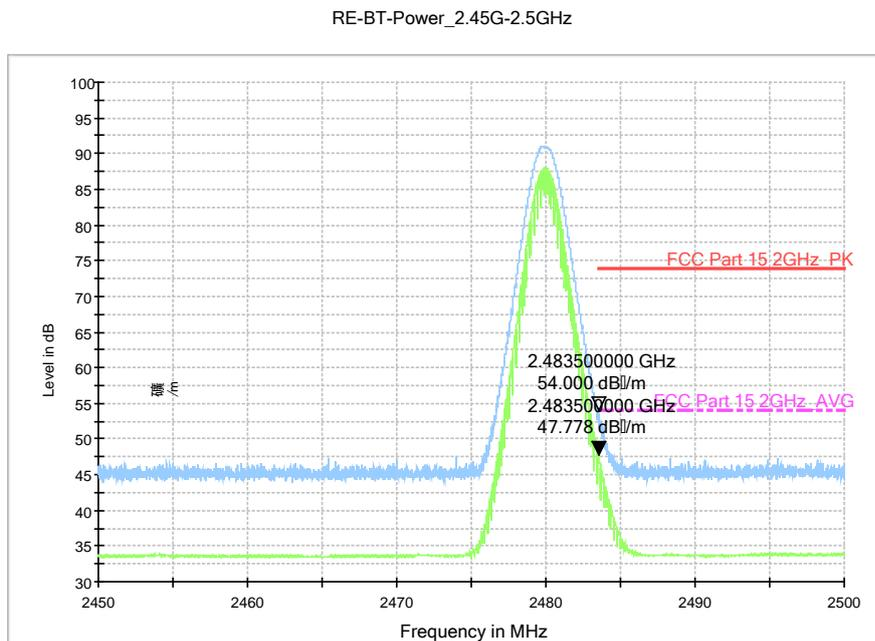
Fig.58. Radiated emission (Power):  $\pi/4$  DQPSK, high channel
