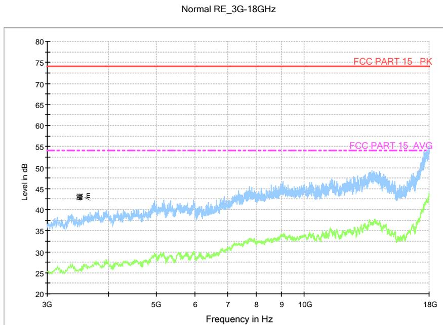
Fig.44. Radiated emission: GFSK, Channel 39, 3 GHz - 18 GHz
