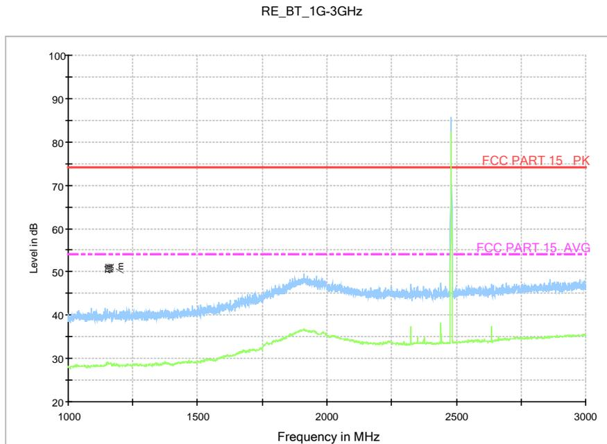
Fig.55. Radiated emission:  $\pi/4$  DQPSK, Channel 78, 1 GHz - 3 GHz
