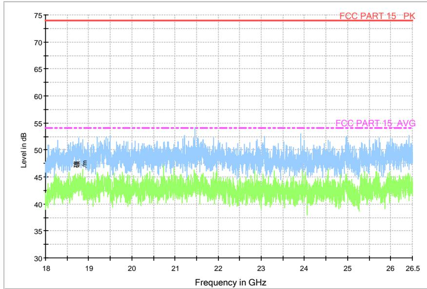
Fig.49. Radiated emission: GFSK, 18 GHz - 26 GHz
