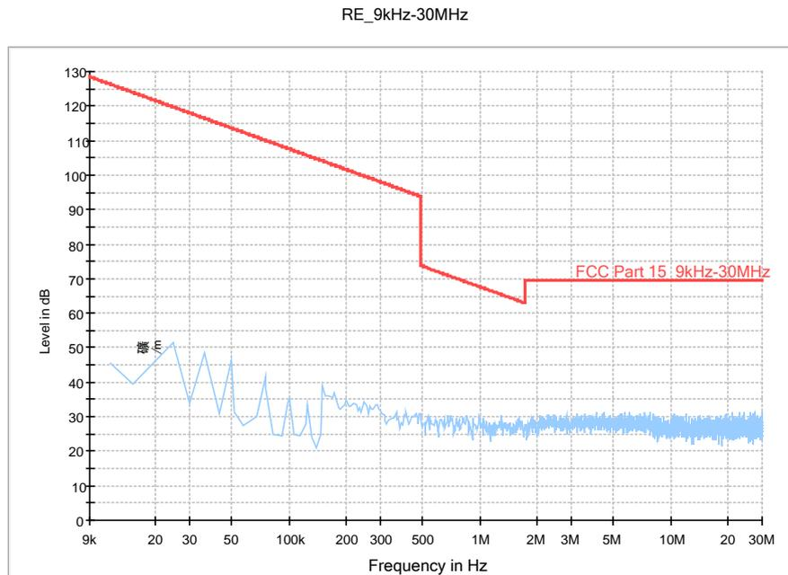
Fig.41. Radiated emission: GFSK, Channel 39, 9 kHz - 30 MHz
