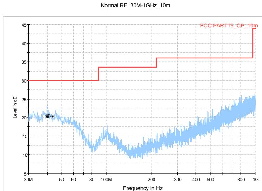
Fig.52. Radiated emission:  $\pi/4$  DQPSK, Channel 39, 30 MHz - 1 GHz
