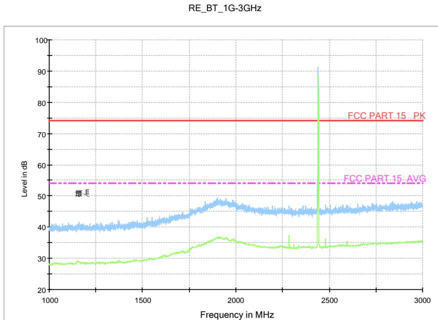
Fig.53. Radiated emission:  $\pi/4$  DQPSK, Channel 39, 1 GHz - 3 GHz
