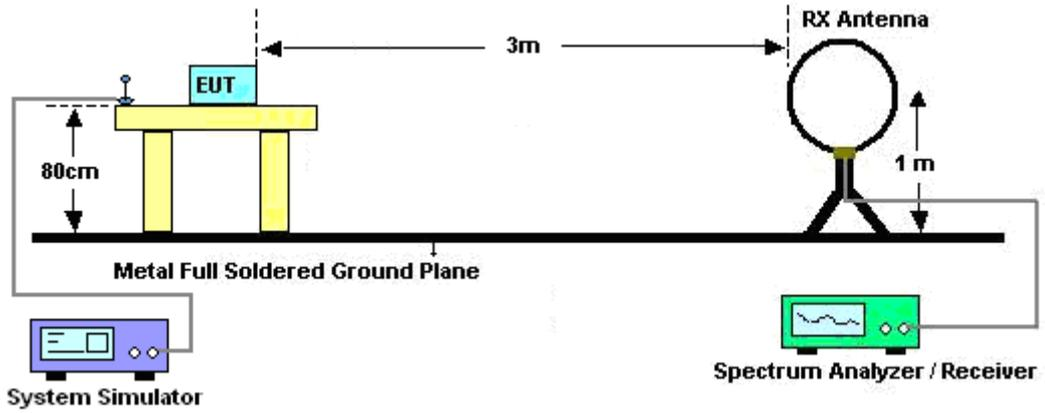
For radiated emissions from 30MHz to 1GHz
