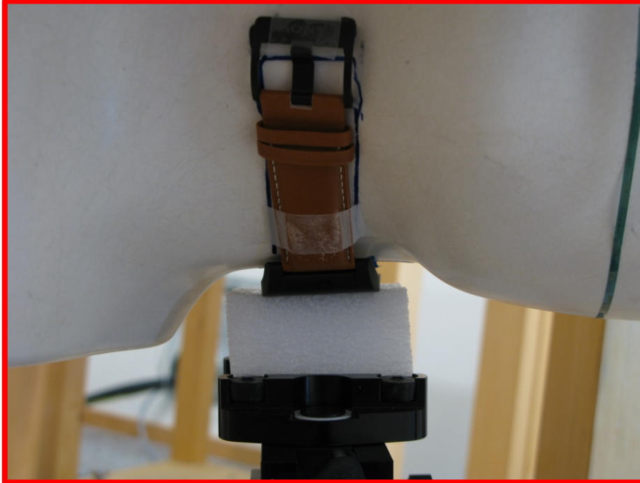
Photograph I2.1 – Back of the Device Placed Against the Phantom Special Neck Position / 1294-5702 (Carrier) and 1276-4067 (Leather Band)
