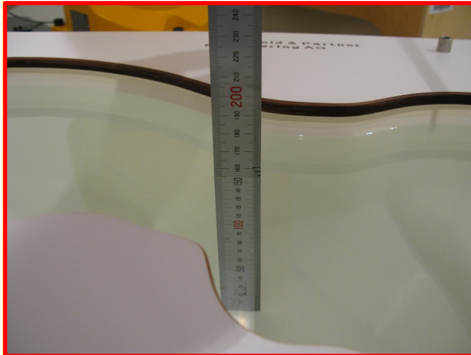
Photograph I3.1 – MSL2450V2 LB000182AA Fluid Level at Test Position 2015-01-15
