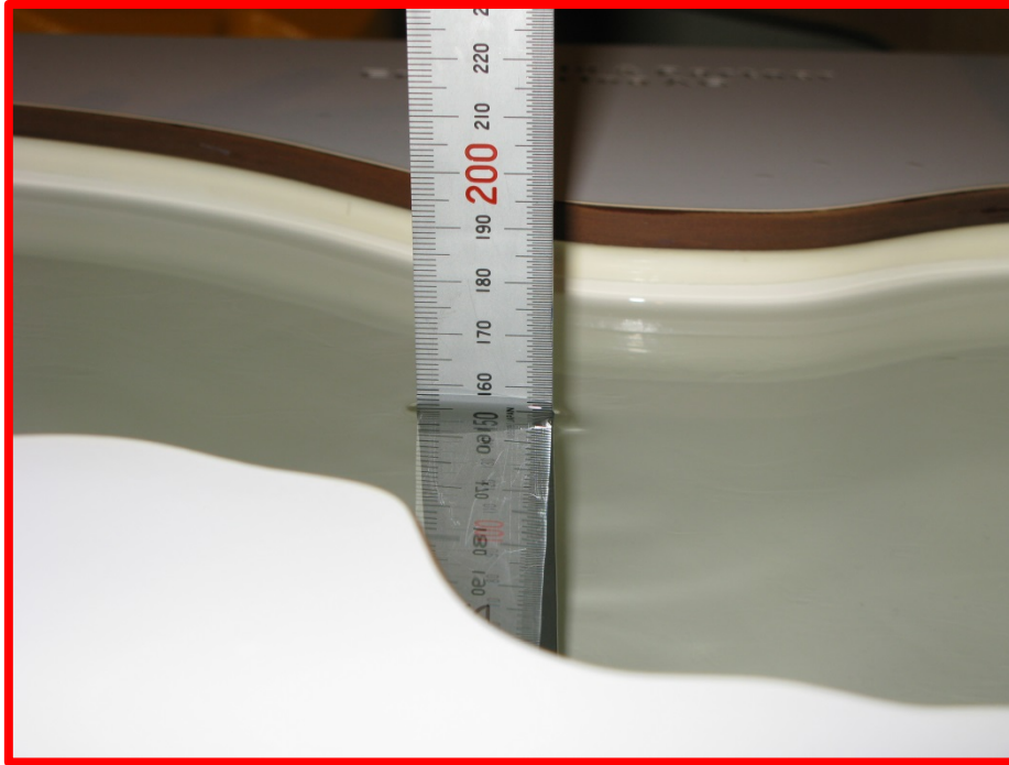
Photograph I3.1 – MSL2450V2 LB000182AA Fluid Level at Test Position 2014-08-20
