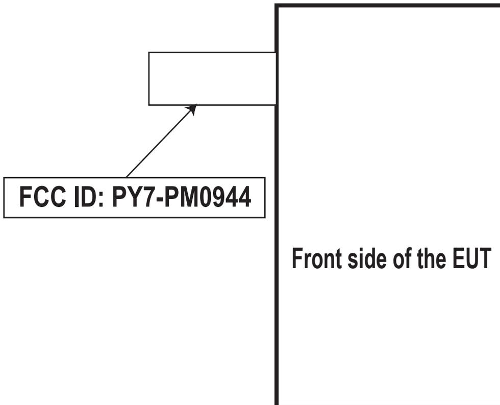
The FCC ID is not on the exterior of the device but labelling meets the conditions allowed in KDB 784748 for the label to be placed in a user accessible area:
