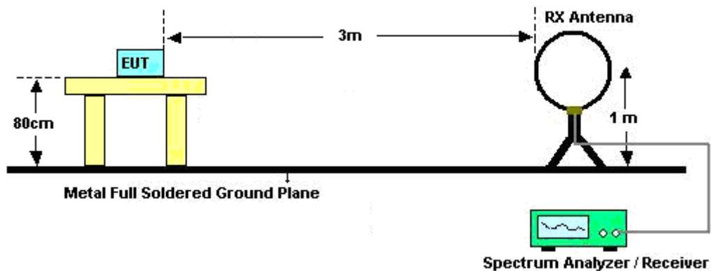
For radiated emissions from 30MHz to 1GHz
