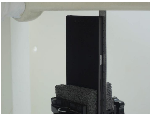
Top Side, Test Separation 10 mm
