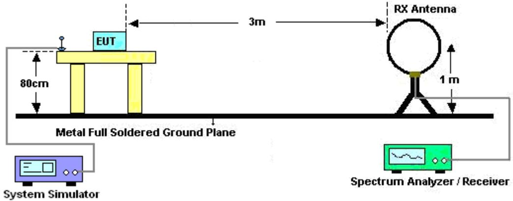
For radiated emissions from 30MHz to 1GHz
