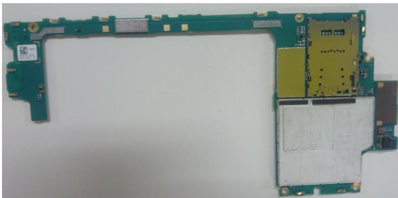
Internal PWB with Shield cases (Front-side)
