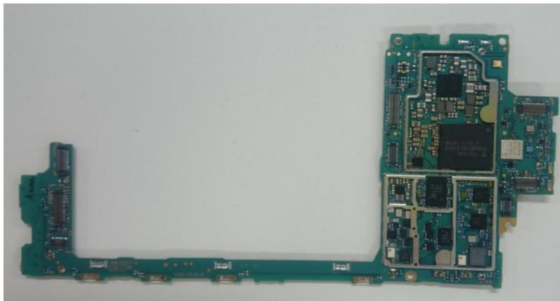
**Internal PWB without Shield cases (Rear-side)**
