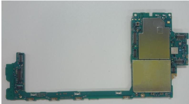
**Internal PWB with Shield cases (Rear-side)**
