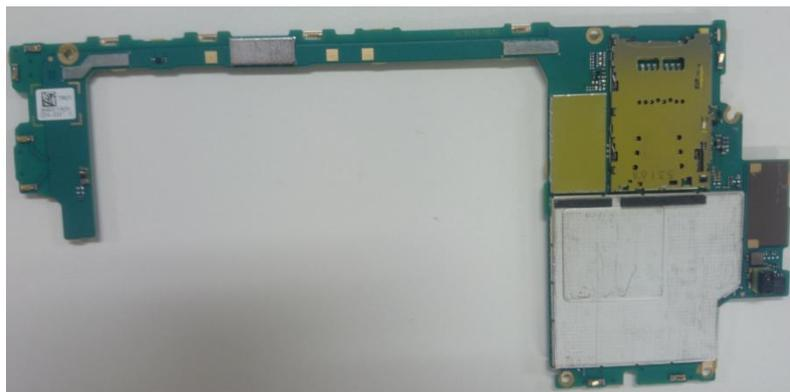
Internal PWB with Shield cases (Front-side)
