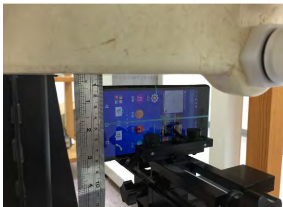
Fig.15 EUT left to flat phantom
