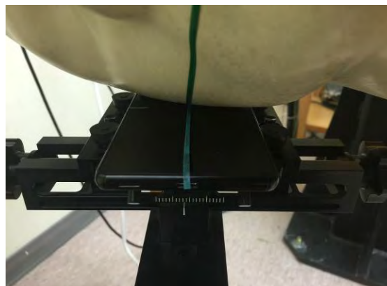
Fig.3 Right Head Section / Cheek-Touch Position
