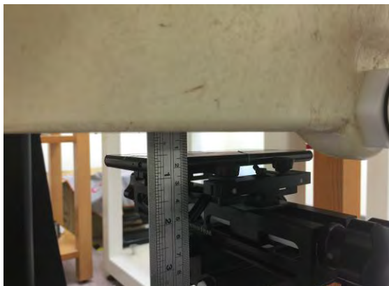
Fig.7 EUT front side to flat phantom
