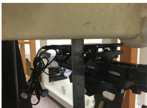
Fig.11 EUT back with headset to flat phantom
