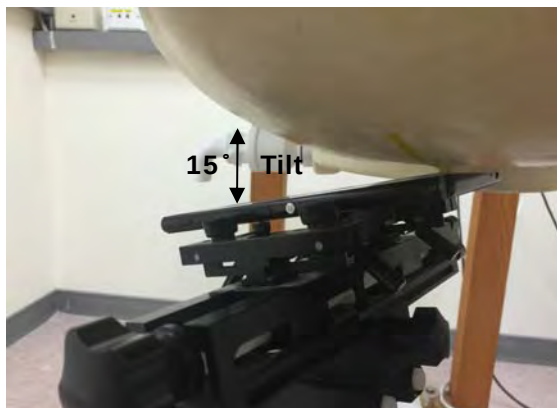
Fig.6 Left Head Section / Ear-Tilt Position(15°)
