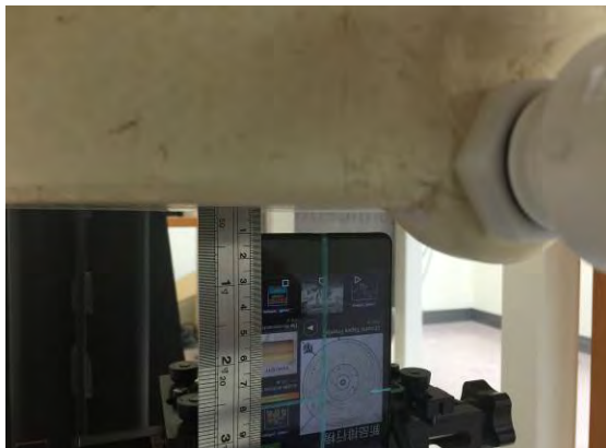
Fig.13 EUT bottom to flat phantom
