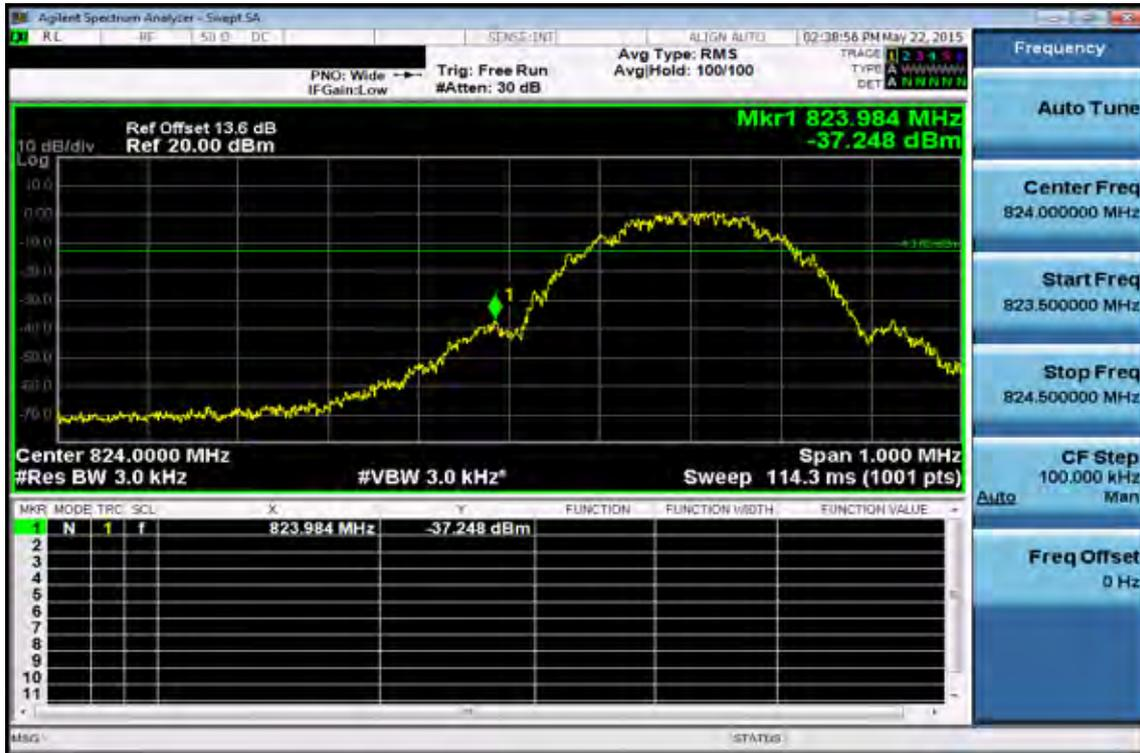
**Band edge emission at antenna terminals – EDGE 850 Channel Highest**
