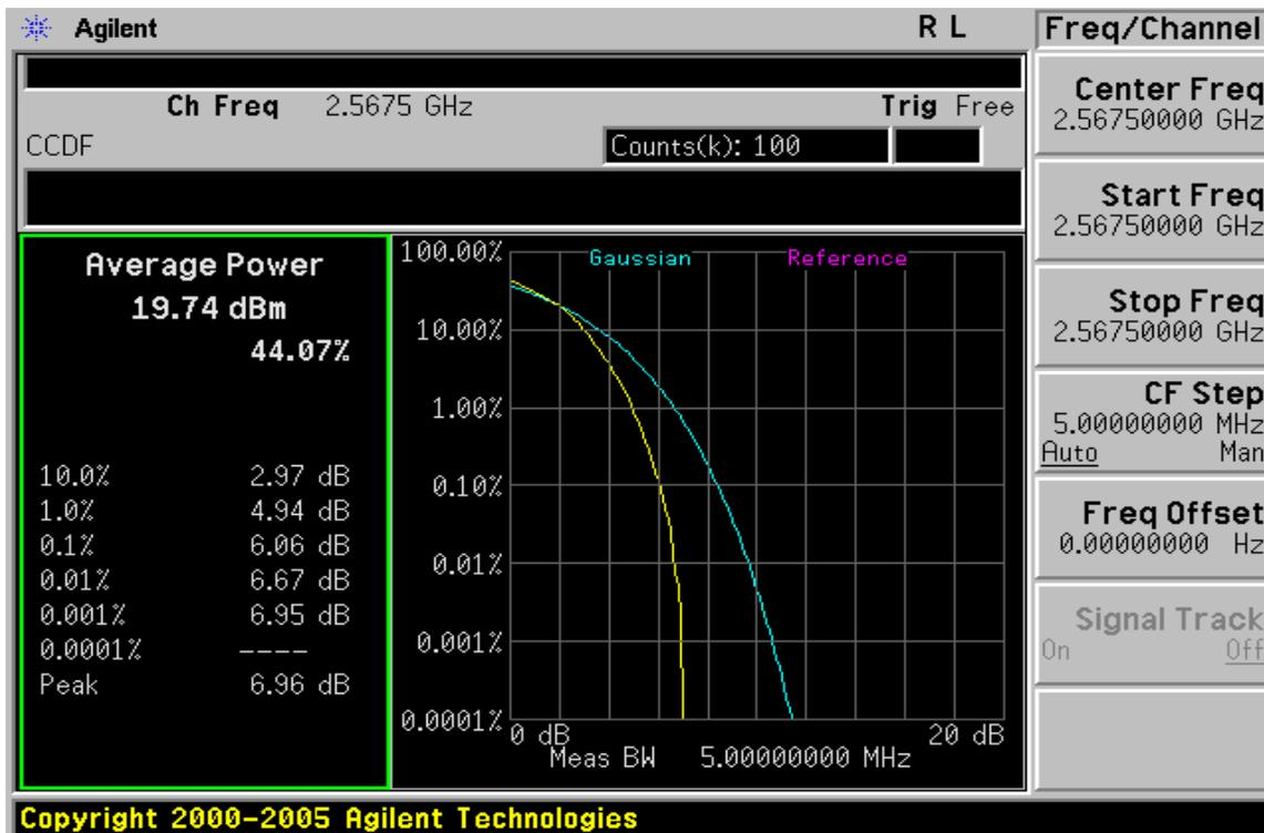
**10MHz BW LTE-Band 7(16QAM Number: 50 Offset: 0) Channel Low**
