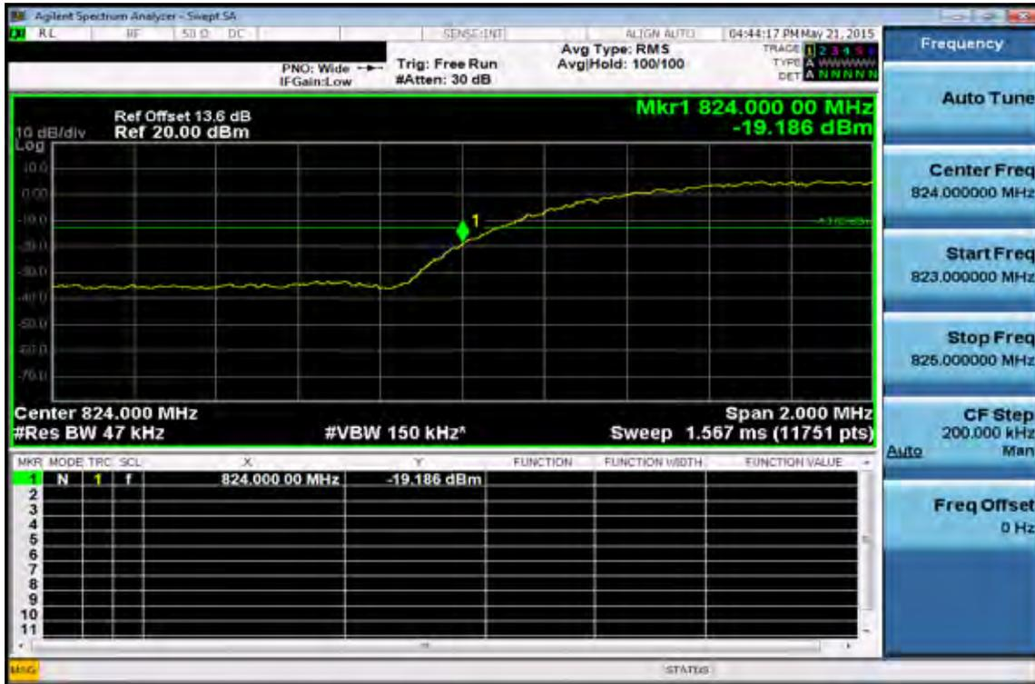
**Band edge emission at antenna terminals – WCDMA V Channel Highest**
