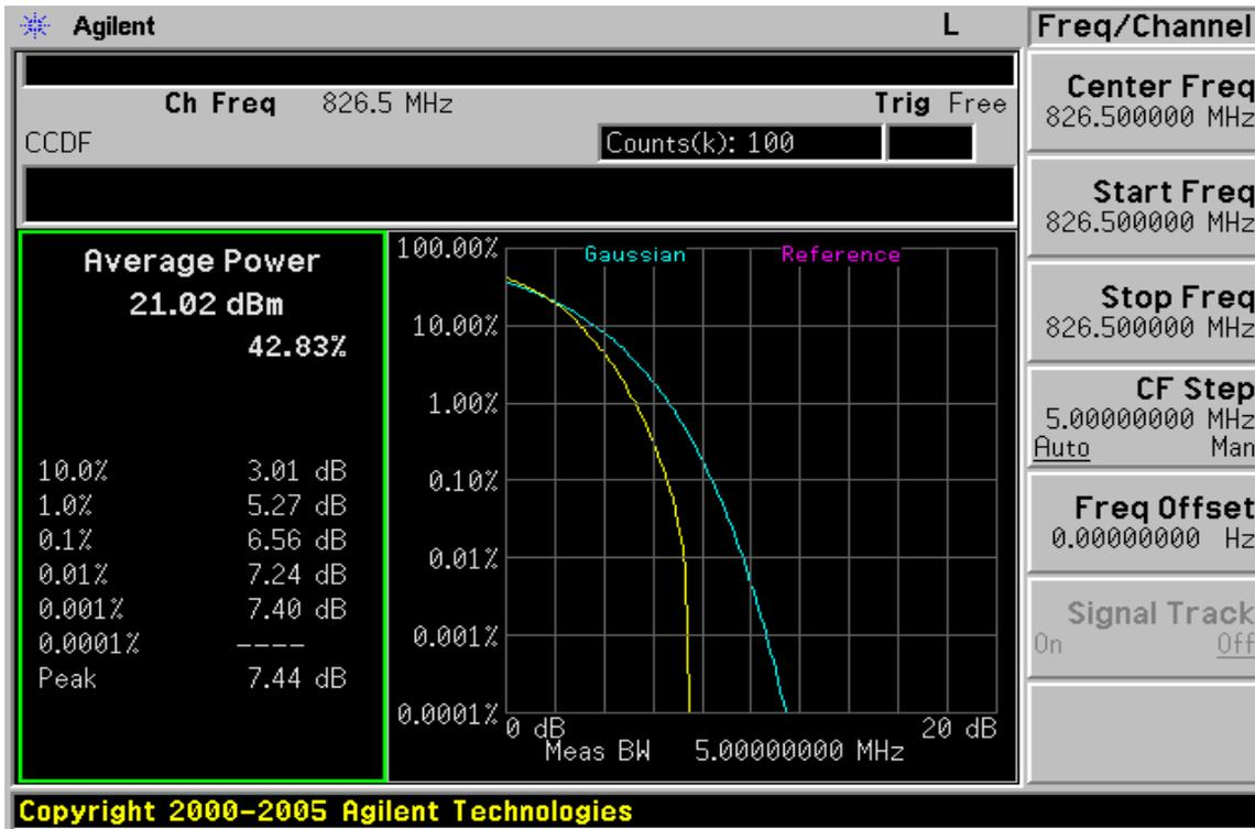
**5MHz BW LTE-Band 5(16QAM Number: 25 Offset: 0) Channel Mid**
