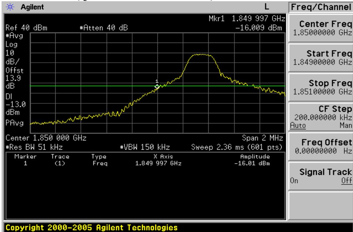
**Band edge emission at antenna terminals –5MHz BW LTE-Band 2
