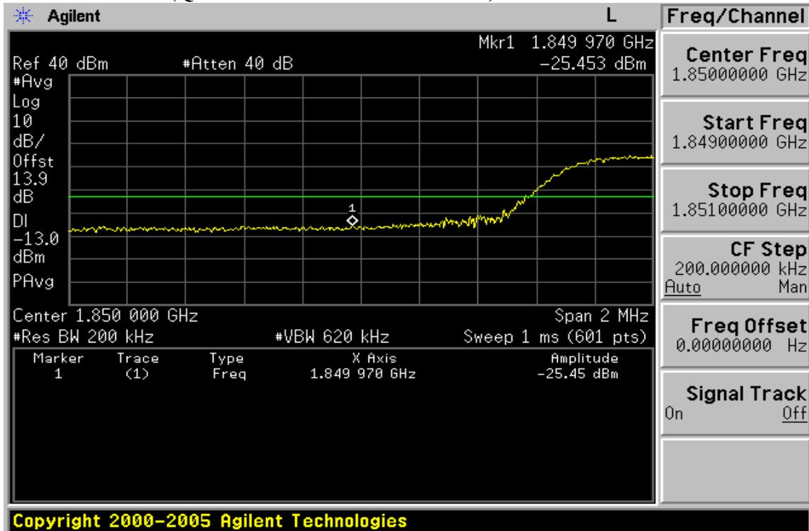
**Band edge emission at antenna terminals –15MHz BW LTE-Band 2
