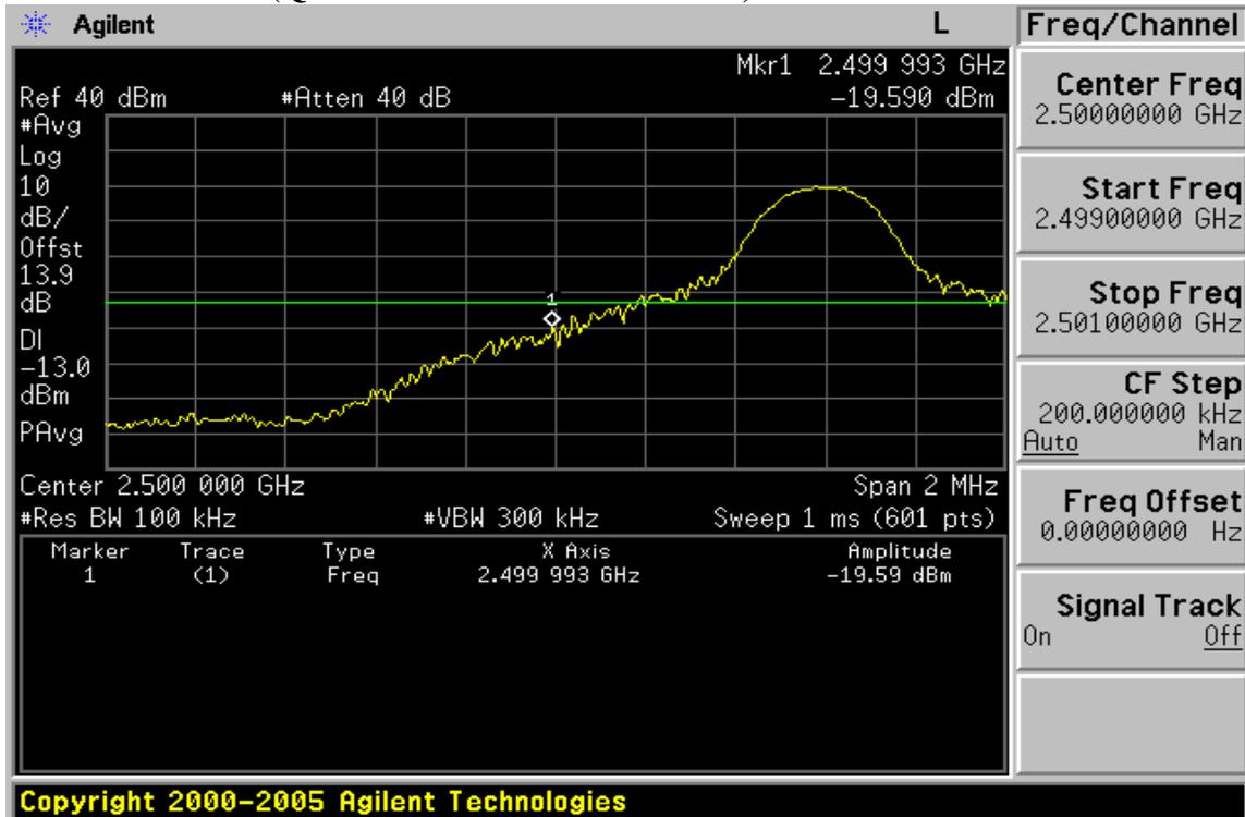
**Band edge emission at antenna terminals –10MHz BW LTE-Band 7
