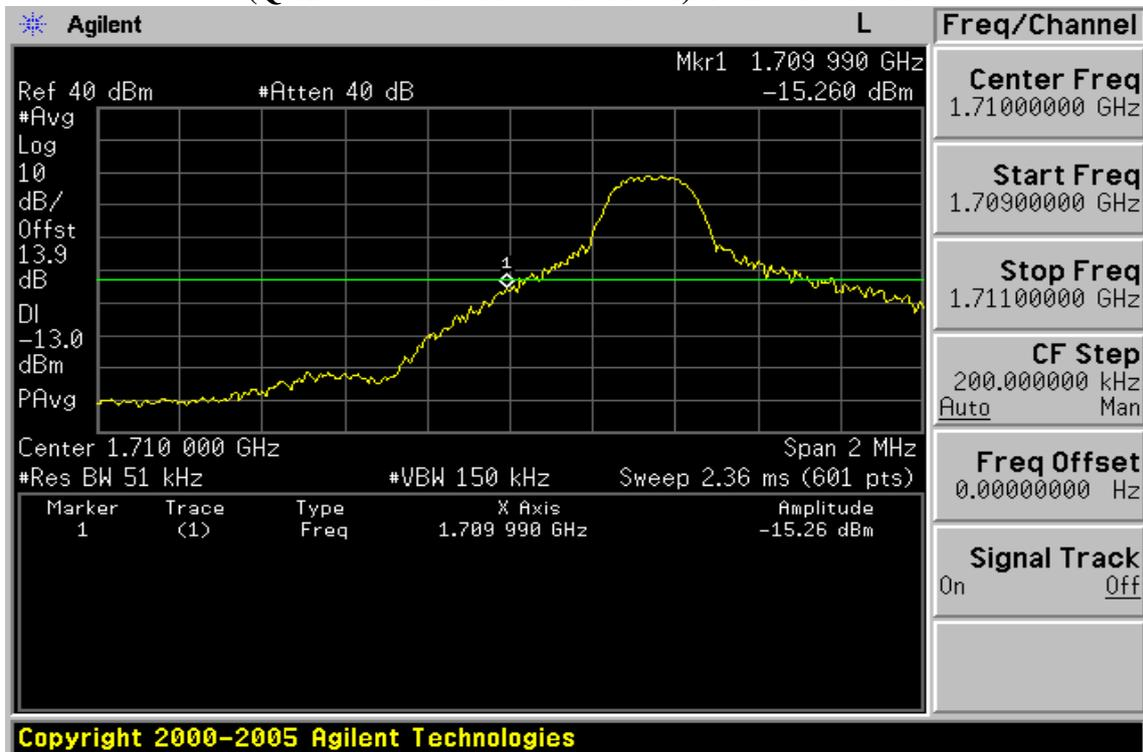
**Band edge emission at antenna terminals –5MHz BW LTE-Band 4
