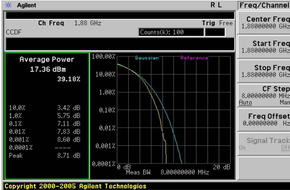
**20MHz BW LTE-Band 2(16QAM Number: 100 Offset: 0) Channel High**
