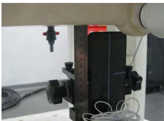
Fig.13 EUT bottom with headset to flat phantom
