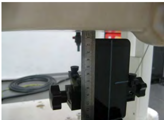
Fig.12 EUT bottom to flat phantom
