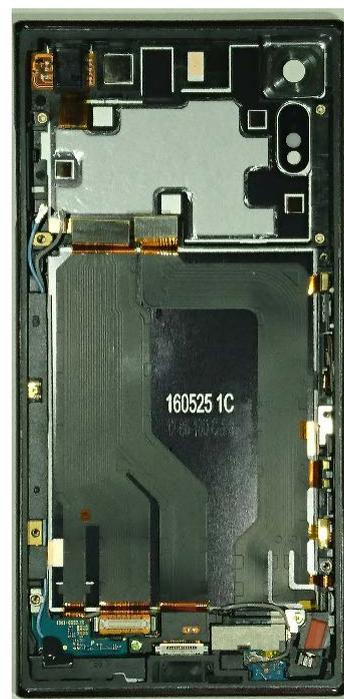
**Internal PWB with/without Shield cases**
