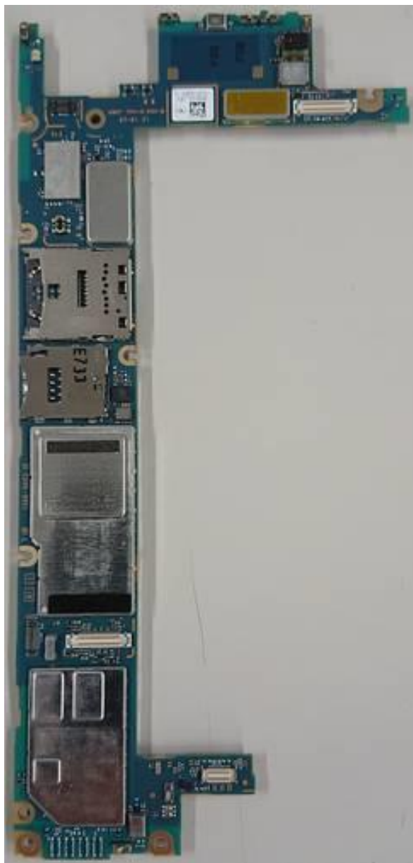
Internal PWB with Shield cases (Front-side)
