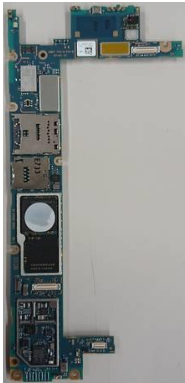
Internal PWB without Shield cases (Front-side)
