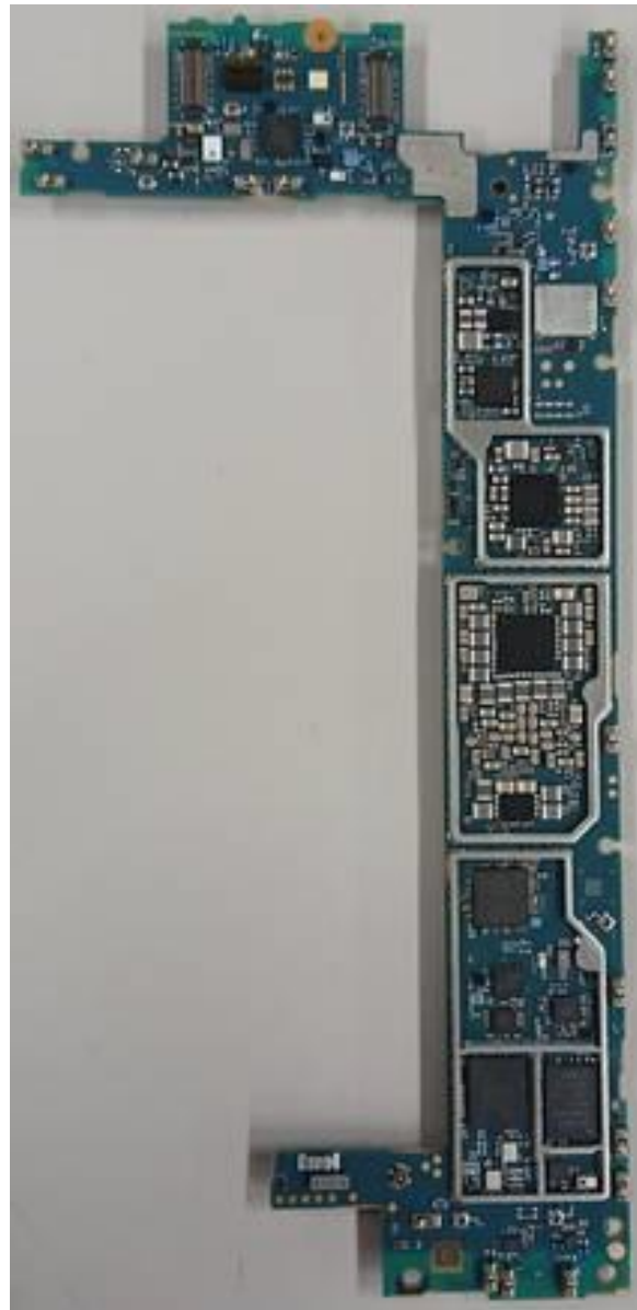
Internal PWB without Shield cases (Rear-side)
