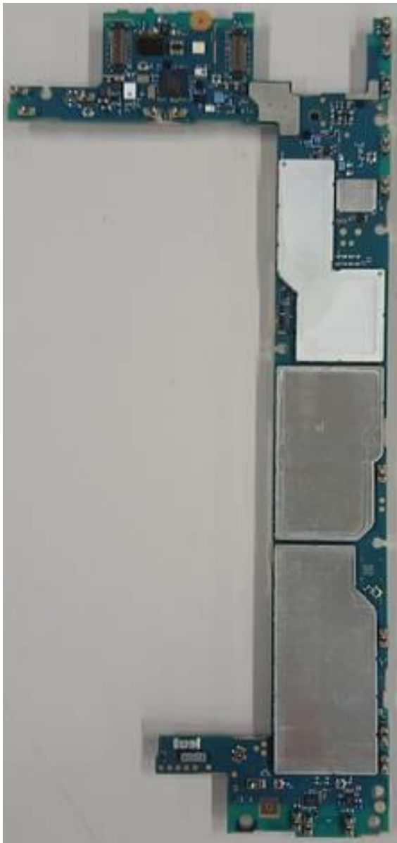
Internal PWB with Shield cases (Rear-side)
