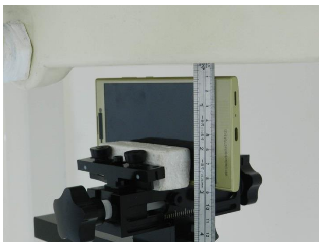
Right Side, Test Separation 10 mm
