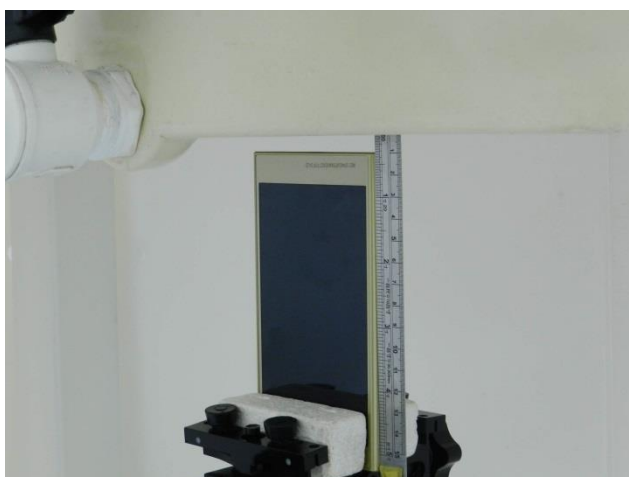
Bottom Side, Test Separation 10 mm
