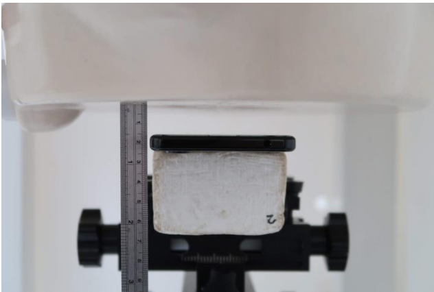
Front, Test Separation 15 mm
