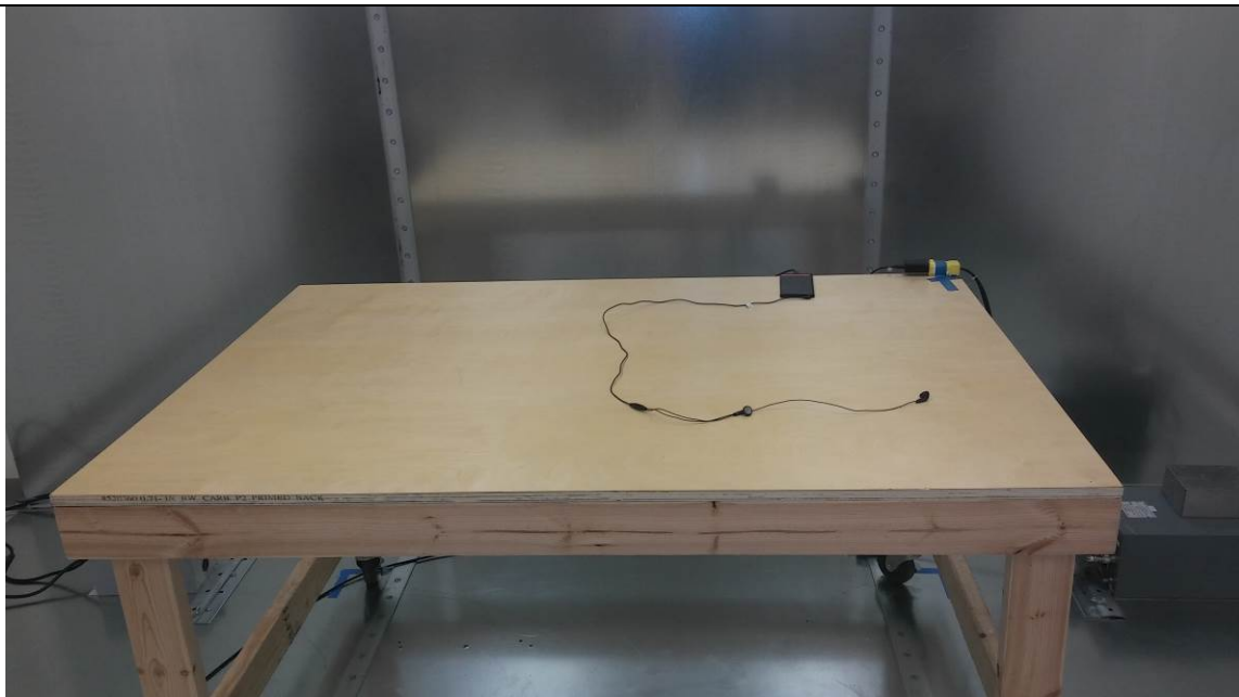
Figure 1 Test Setup for Conducted Emissions - Charger
