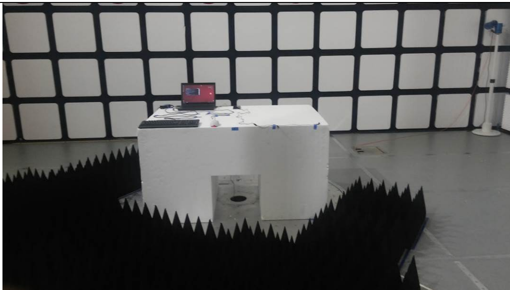
Figure 10 Test setup for Radiated Emissions > 1GHz Sync
