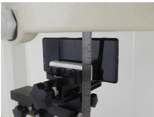
Right Side, Test Separation 10 mm
