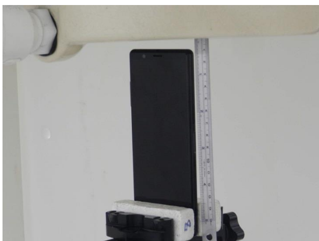
Top Side, Test Separation 10 mm
